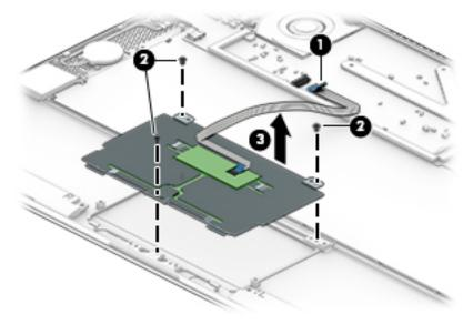
Reverse this procedure to install the TouchPad board.
