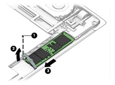
Reverse this procedure to install the solid-state drive.
