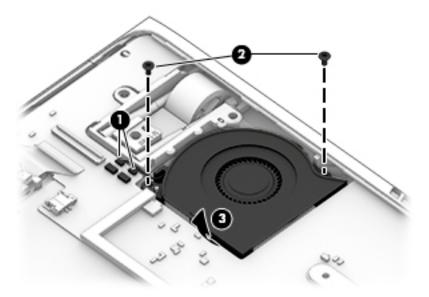
2. To remove the right fan, disconnect the fan cables from the system board (1), remove the two Phillips PM2.0×3.0 screws (2), and then lift the fan at an angle (approximately 45 degrees) and pull it out from under the edge of the computer (3).
