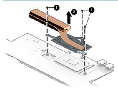
NOTE: The thermal material must be thoroughly cleaned from the surfaces of the heat sink and the system board each time the heat sink is removed. Replacement thermal material is included with the heat sink and system board spare part kits. Thermal paste is used on the heat sink (1) and on the system board (2) as shown in the following image.
