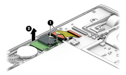
NOTE: If the WLAN antennas are not connected to the WLAN module, the protective sleeve should be installed on the antenna connectors, as shown in the following illustration.
