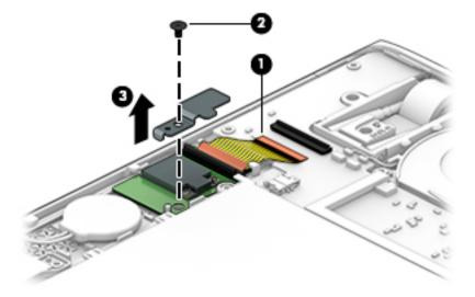
4. Disconnect the WLAN antenna cables (1) from the WLAN module terminals.
