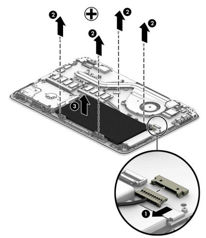
Reverse this procedure to install the battery.
