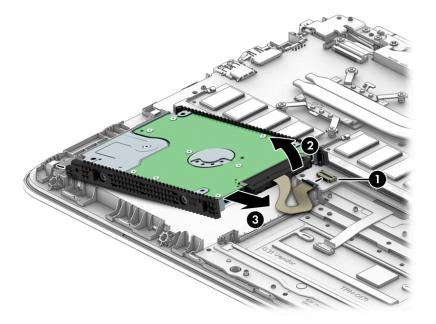
4. If it is necessary to replace the hard drive bracket, remove the left and right brackets (1).
