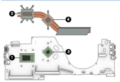
Thermal material is used on the processor (1) and the heat sink section (2) that services it. The following illustration shows the thermal material locations on a computer model equipped with a graphics subsystem with UMA memory.
