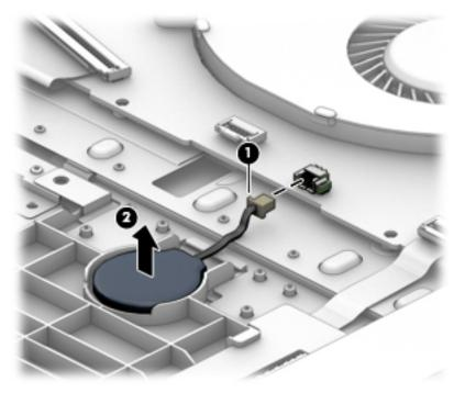
3. Remove the RTC battery.
