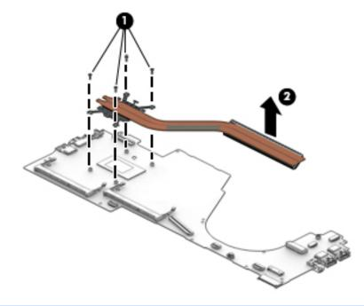
NOTE: The thermal material must be thoroughly cleaned from the surfaces of the heat sink and the system board each time the heat sink is removed.
