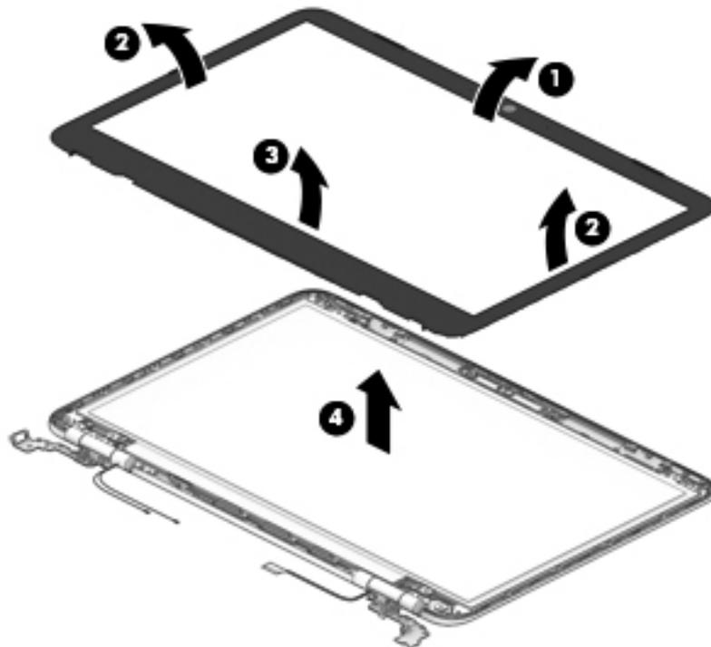
7. If it is necessary to replace the display panel:
