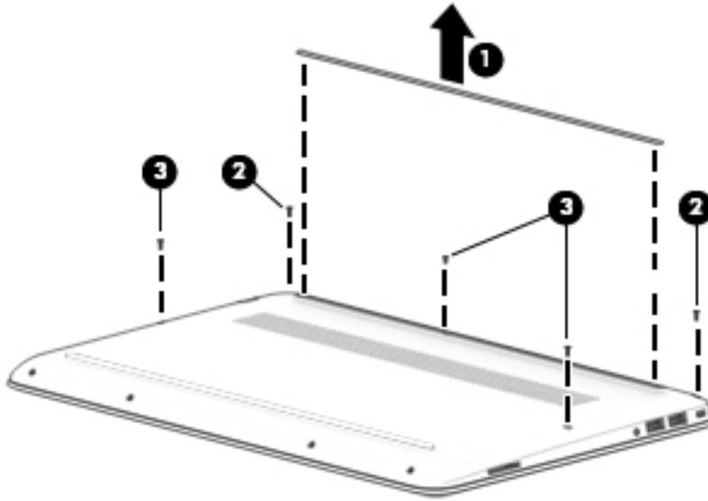
5. Remove the four Phillips M2.0×5.7 screws that secure the bottom cover to the computer.
