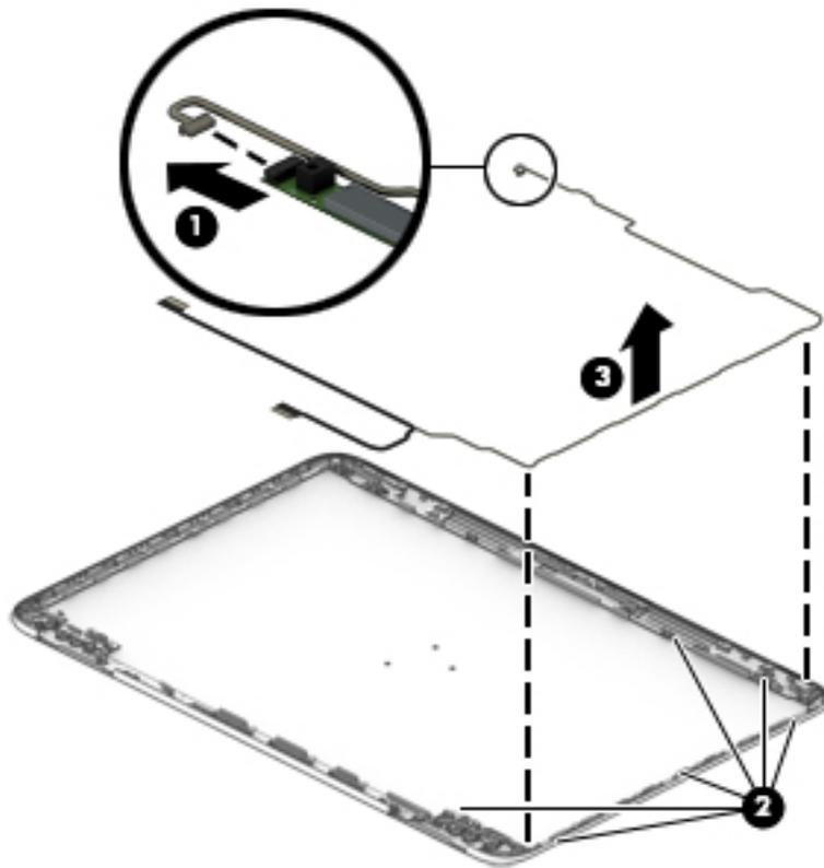
9. If it is necessary to replace the webcam/microphone module:
