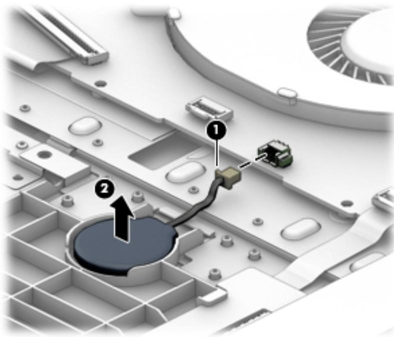
3. Remove the RTC battery.
