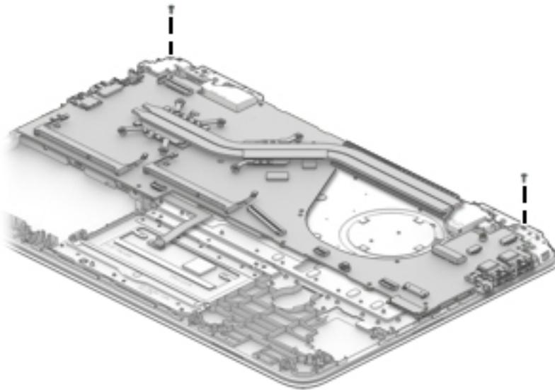
3. Release the system board **(1)** by lifting the front edge and swinging it up and back until it rests upside down behind the computer.
