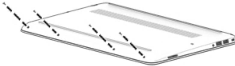
6. Insert a case utility tool **(1)** or similar plastic, flat-edged tool between the bottom cover and the computer.
