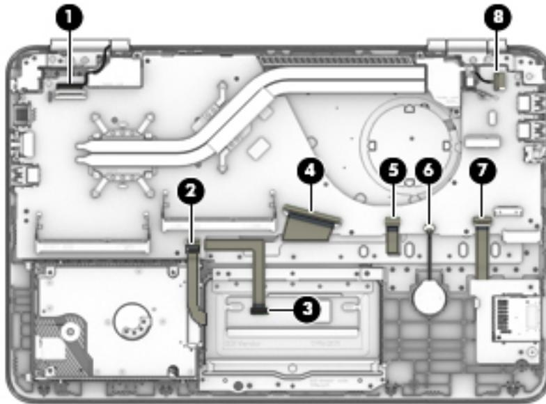
2. Remove the two Phillips PM2.0×5.7 screws that secure the system board to the keyboard/top cover.
