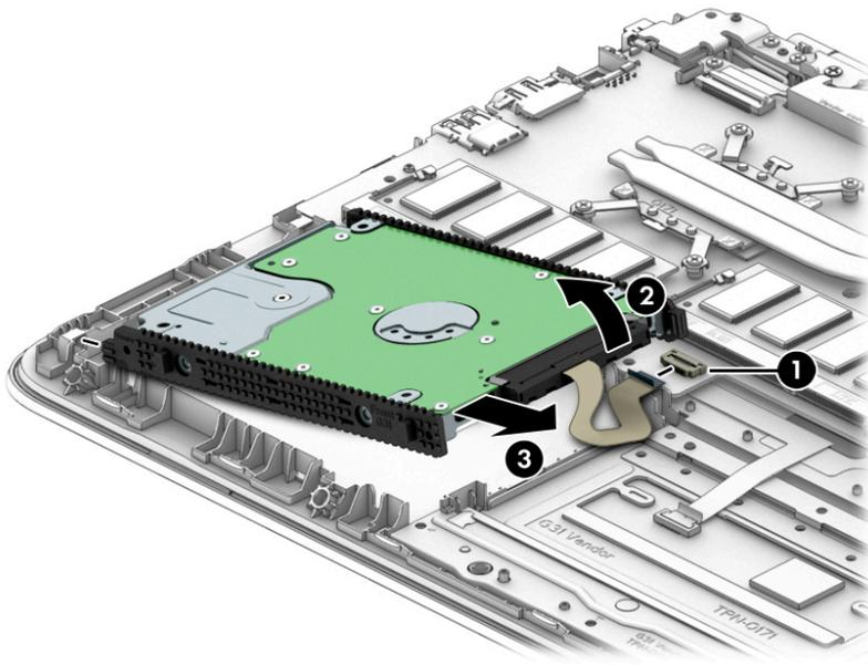
4. If it is necessary to replace the hard drive bracket, remove the left and right brackets **(1)**.
