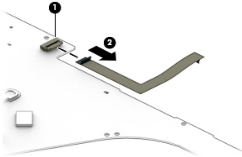
Reverse this procedure to install the TouchPad cable.
