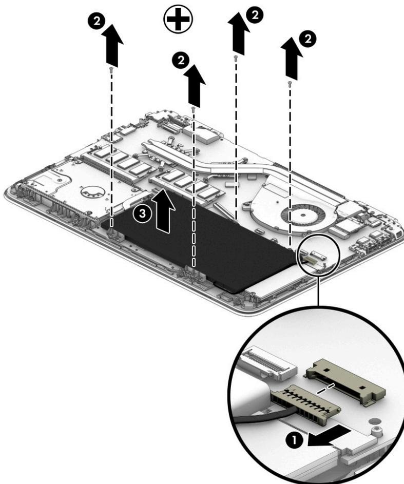
Reverse this procedure to install the battery.
