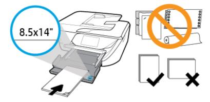
Make sure the stack of paper is aligned with the appropriate paper size lines on the front of the tray. Besides, make sure the stack of paper does not exceed the stack height marking on the edge of the tray.
