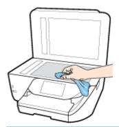
**CAUTION:** Use only glass cleaner to clean the scanner glass. Avoid cleaners that contain abrasives, acetone, benzene, and carbon tetrachloride, all of which can damage the scanner glass. Avoid isopropyl alcohol because it can leave streaks on the scanner glass.
