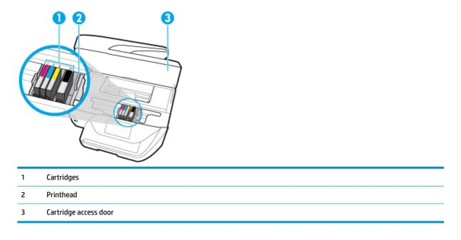
NOTE: Cartridges should be kept in the printer to prevent possible print quality issues or printhead damage. Avoid removing supplies for extended periods of time. Do not turn the printer off when a cartridge is missing.
