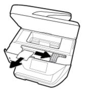
**b.** Move the carriage to the far left of the printer, and do the same as in the previous step to remove any torn pieces of paper.
