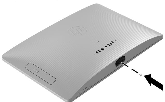
5. Align the stand with the holes on the bottom of the computer, and then tighten the two captive screws.
