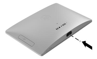
2. Insert the drive cage into the computer (1), replace the Phillips screw (2), and then connect the drive cable to the drive (3).
