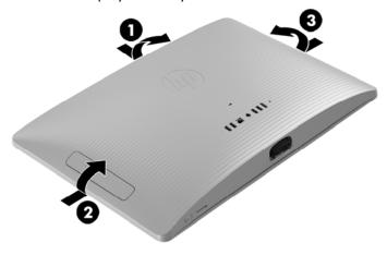
6. To avoid damaging the cable that connects the system board to the rear cover, carefully lift the bottom edge of the cover, and then rotate the cover until it rests upside down next to the display assembly.
