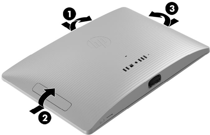
6. To avoid damaging the cable that connects the system board to the rear cover, carefully lift the bottom edge of the cover, and then rotate the cover until it rests upside down next to the display assembly.
