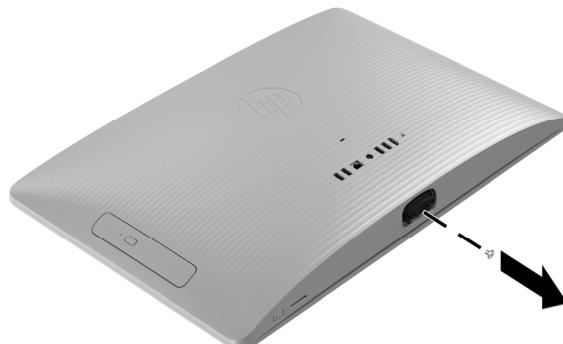
5. Starting with the gap at the top of the cover, pry the top (1), left edge (2), and right edge (3) of the cover away from the display assembly in the order shown.
