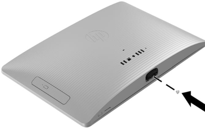
6. Align the stand with the holes on the bottom of the computer, and then tighten the two captive screws.
