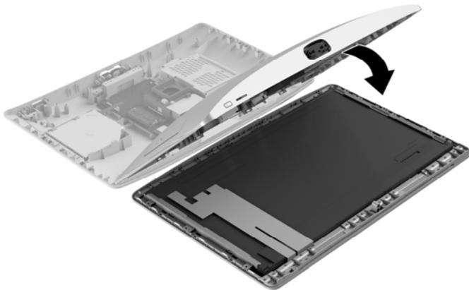
4. Align the cover with the computer and press it down until it snaps into place.
