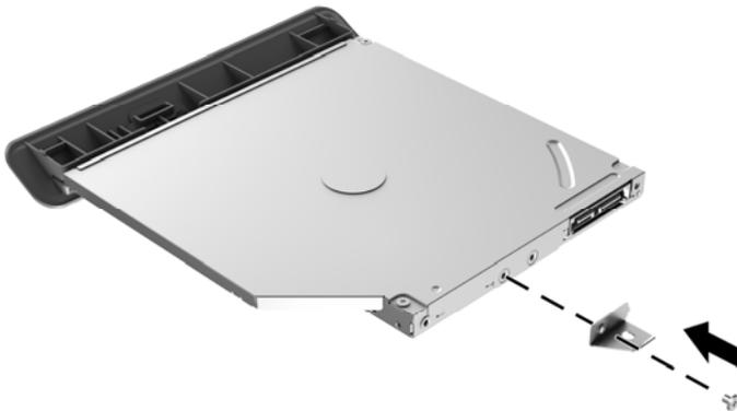
2. Slide the drive into the computer (1), replace the Phillips screw (2), and then connect the cable to the drive (3).
