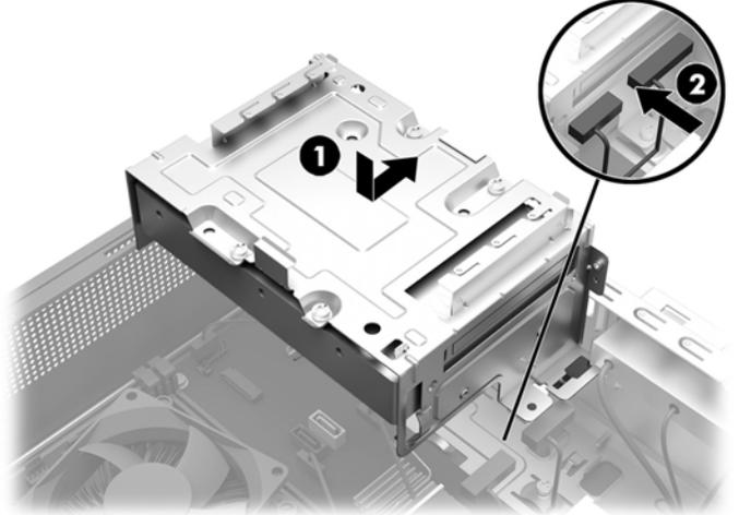
3. Replace the three Phillips screws that secure the drive cage to the front of the computer and the Phillips screw that secures the drive cage to the inside of the computer.
