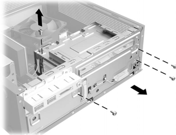
6. Disconnect the data and power cables from the rear of the hard drive (1), and then slide the drive cage away from the front and lift it out of the computer (2).
