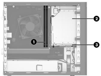
5. Remove the three Phillips screws that secure the drive cage to the front of the computer and the Phillips screw that secures the drive cage to the inside of the computer.
