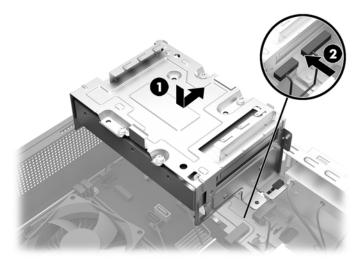
Replace the bezel by inserting the tabs at the bottom of the bezel into the slots in the front of the computer (1), and then rotating the bezel upward and snapping it into place (2).
