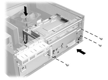
2. Insert the drive cage into the computer (1), and then connect the power and data cables to the back of the hard drive (2).
