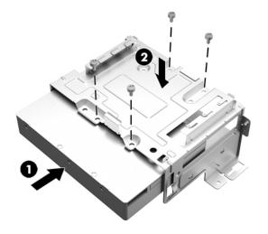
3. Replace the three Phillips screws that secure the drive cage to the front of the computer and the Phillips screw that secures the drive cage to the inside of the computer.
