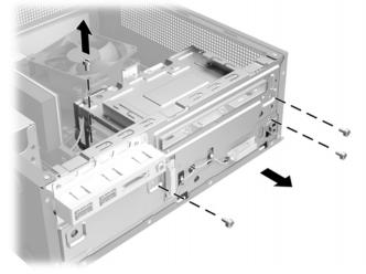
7. Remove the four Phillips screws that secure the hard drive to the hard drive cage (1), and then slide the hard drive out of the hard drive cage (2).
