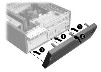
5. Position the access panel on the computer and slide it into place (1). Tighten the captive screw in the rear of the cover (2).
