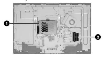
7. Spread the two retention clips outward (1) until the memory module tilts up at a 45-degree angle. Remove the module (2). Use the same procedure to remove both memory modules.
