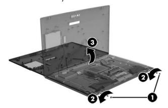
6. Remove the five Phillips screws that secure the system board cover (1), and then lift the cover off the computer (2).
