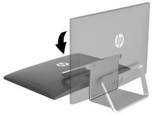
4. To remove the rear cover, remove the two screw covers (1) and two Phillips screws (2) located in the bottom of the cover. Lift off the cover, and then place it upside down next to the computer (3). The optical drive is mounted on the inside of the rear cover, and a cable connects it to the system board.
