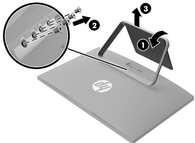
4. To remove the rear cover, remove the two screw covers (1) and two Phillips screws (2) located in the bottom of the cover. Lift off the cover, and then place it upside down next to the computer (3). The webcam cable connects the webcam installed in the rear cover to the system board.
