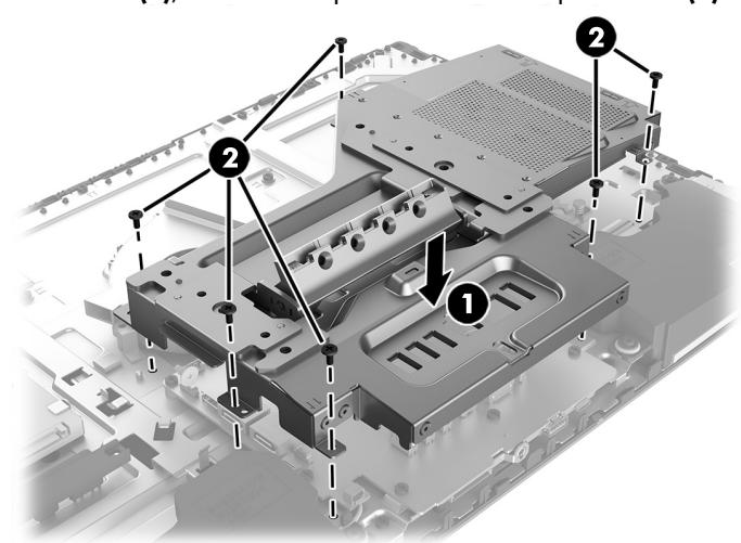
3. Align the rear cover with the computer and press it down until it snaps into place (1). Replace the two Phillips screws (2), and then replace the screw covers (3).
