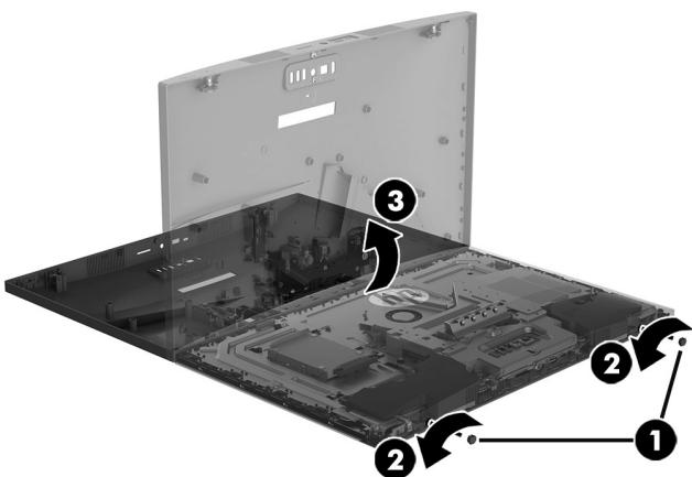
6. Remove the six Phillips screws that secure the system board cover (1), and then lift the cover off the computer (2).
