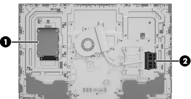
7. Spread the two retention clips outward (1) until the memory module tilts up at a 45-degree angle. Remove the module (2). Use the same procedure to remove both memory modules.
