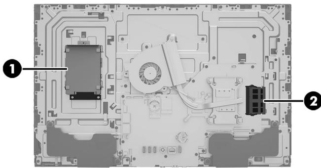
6. To remove the drive from the drive cage, remove the four Phillips screws from the sides of the cage (1), and then slide the drive out of the drive cage (2).
