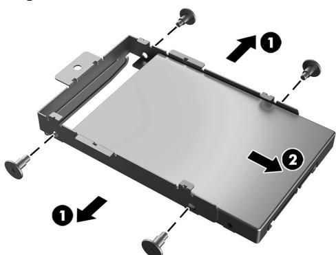
6. Remove the Phillips screw that secures the drive cage (1), pull the cable away from the hard drive (2), and then remove the drive cage from the computer (3).
