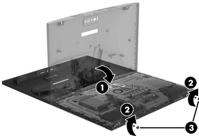
4. Position the top of the stand on the computer (1), and then replace the four hex screws (2). Rotate the stand downward (3).
