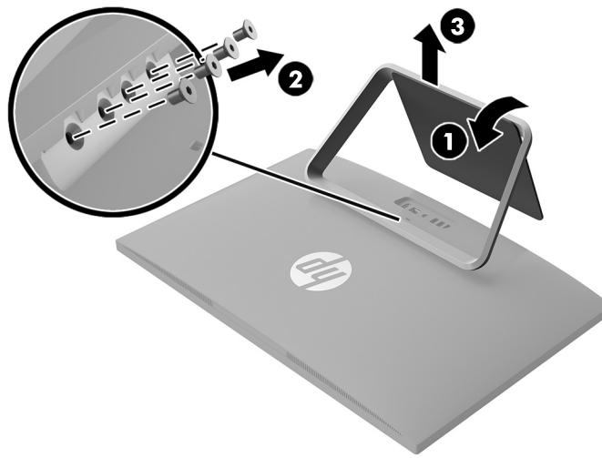
4. To remove the rear cover, remove the two screw covers (1) and two Phillips screws (2) located in the bottom of the cover. Lift off the cover, and then place it upside down next to the computer (3). The webcam cable connects the webcam installed in the rear cover to the system board.
