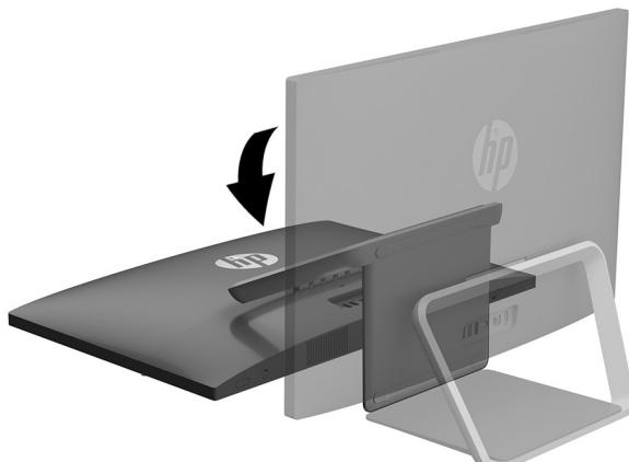
3. To remove the stand, rotate it upward (1), remove the four hex screws (2), and then lift the stand up and off the computer (3).
