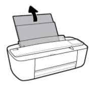
2. Insert a stack of paper into the input tray with the short edge down and the print side up, and slide the stack of paper down until it stops.
