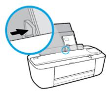
4. Pull out the output tray and the output tray extender, and then lift the paper catch.
