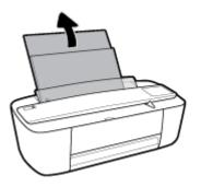
2. Insert one or more envelopes into the far-right side of the input tray and slide the stack of envelopes down until it stops. The side to be printed on should face up.
