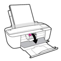
**b.** Press down to release the cartridge, and then pull it toward you out of the slot.
