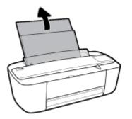
2. Insert a stack of photo paper into the far-right side of the input tray with the short edge down and the print side up, and slide the stack of paper down until it stops.
