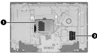
7. To remove the hard drive from the drive cage, remove the four Phillips screws from the sides of the cage (1), and then lift the drive out of the drive cage (2).
