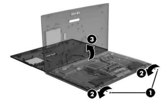
Remove the Phillips screw that secures the drive cage (1), pull the cable away from the hard drive (2), and then remove the drive cage from the computer (3).
