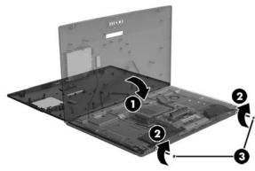
2. Insert the drive cage into the computer and slide the drive cage until it is seated (1). Attach the cable to the hard drive (2), and then replace the Phillips screw (3).
