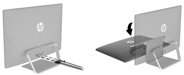
3. To remove the stand, rotate it upward (1), remove the four hex screws (2), and then lift the stand up and off the computer (3).
