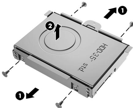
6. Remove the Phillips screw that secures the drive cage (1), pull the cable away from the hard drive (2), and then remove the drive cage from the computer (3).
