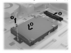
7. To remove the drive from the drive cage, remove the four Phillips screws from the sides of the cage (1), and then slide the drive out of the drive cage (2).
