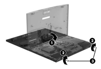
2. Insert the drive cage into the computer and slide the drive until seated (1). Attach the cable to the drive (2), and then replace the Phillips screw (3).
