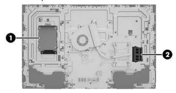
Remove the Phillips screw that secures the drive cage
