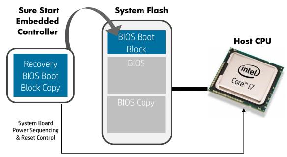
Figure 2 Firmware Integrity Verification Process
