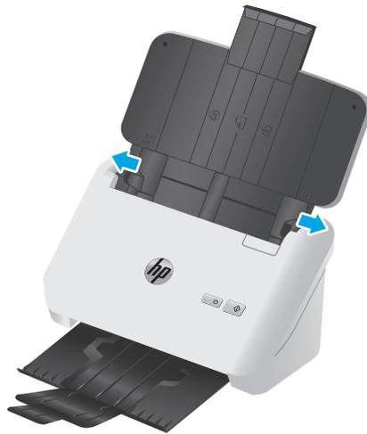
When scanning small originals such as checks, it is especially important that the paper guides fit snugly against the edges of the original yet not restrict paper feeding.
