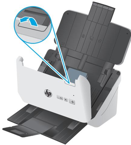
3. Release the pickup roller cover tab.
