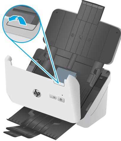
3. On the rear of the open document feeder, use a fingertip to press the tab at the upper right corner of the pickup roller cover, and then forward to open the cover and expose the pickup rollers.
