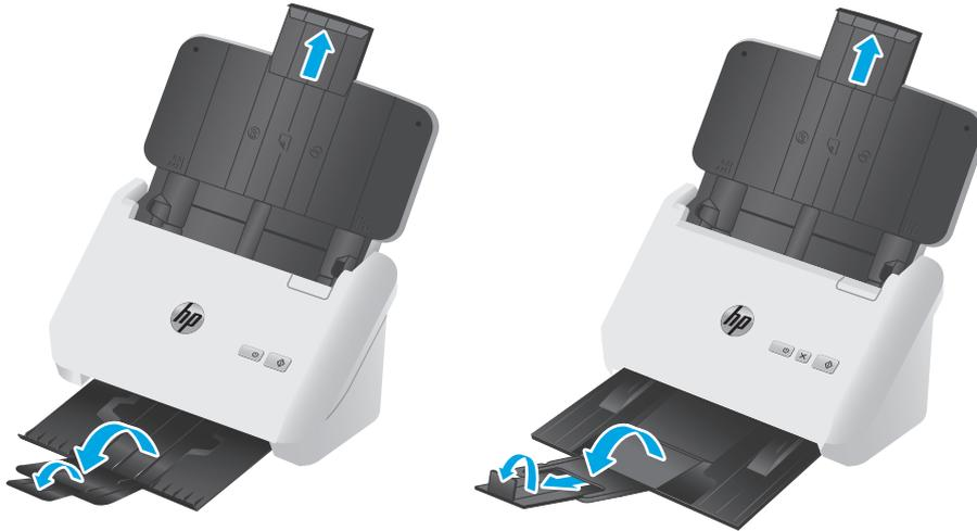
**3000 s3 models:** For the output tray, slide the tray out from underneath the scanner, unfold the first extension, slide the second extension outward, and then rotate the small third tab 90 degrees.
