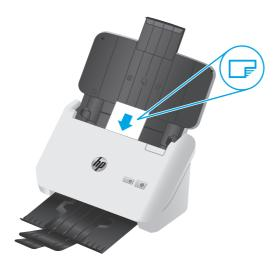
NOTE: To ensure the best scan quality, load rigid or embossed cards in this orientation, and load only one at a time.
