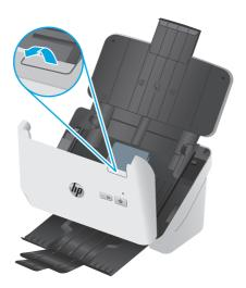
3. Clean the scanning strips with a soft, lint-free cloth that has been sprayed with a mild glass cleaner.
