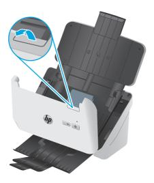
3. Release the pickup roller cover tab.
