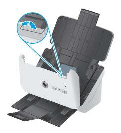
3. Release the pickup roller cover tab.
