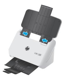
3. 3000 s3 models: Set the output tray small media guide, and disable the multi-feed detection setting.
