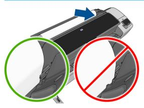
9. Roll the paper into the printer until you feel resistance and the paper flexes slightly. When the printer detects the paper, it feeds it in automatically.
