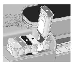
Push the cartridge into the slot until it snaps into position. You should hear a beep and see confirmation that the cartridge has been inserted.
