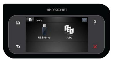
The front panel has a large central area to display dynamic information and icons. On the left and right sides you can see up to six fixed icons at different times. Normally they are not all displayed at the same time.
