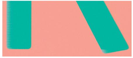
If edges of objects or lines appear to be poorly defined or lighter in density, and you have already set the printquality slider to Quality in the driver dialog, select the custom print-quality options, and try setting the quality level to **Normal**. See Printing on page 50.
