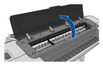
**4.** Find the printhead drop detector beside the stored printhead carriage.
