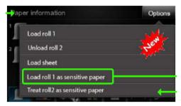
The front panel guides you through a step-by-step process. At the end, you are asked to keep the roll cover open while sensitive-paper mode is active. Apart from that, you can print on the selected roll as usual.
