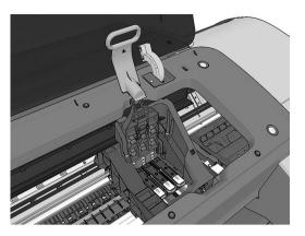
8. To remove a printhead, lift up the blue handle.
