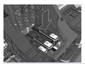
CAUTION: When installing the new printhead there may be some resistance, so you need to press it down firmly but smoothly. You should hear a beep and see confirmation on the front-panel display that the printhead has been inserted. If you have difficulty, see <u>Cannot insert a printhead on page 148</u>.
