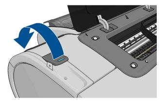
5. Carefully remove any of the jammed paper that you can lift up and out from the top of the printer.
