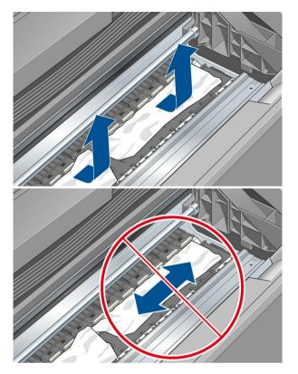
⚠ CAUTION: Do not move the paper sideways, as it could damage the printer.
