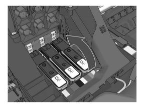
9. Using the blue handle, use steady force to disengage the printhead.
