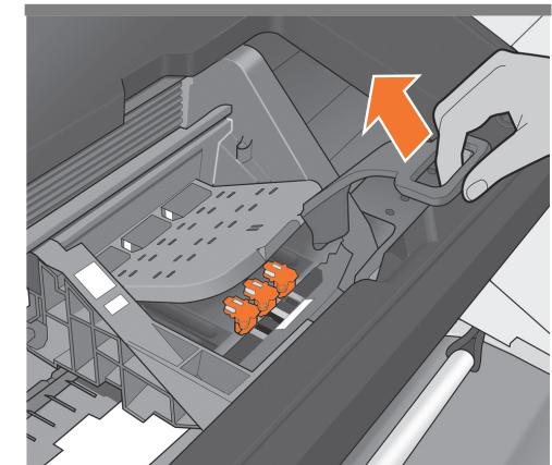
Lift the handle up to open the printhead cover. The front panel prompts you for the next step: removing the printheads. Do not press OK until you have removed all the orange setup printheads.
