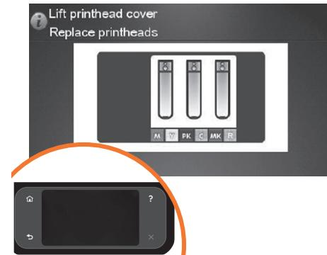
Press the **OK** key on the front panel when you have removed all of the setup printheads. The front panel then prompts you to install the new printheads.
