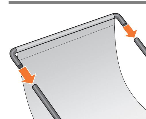
Attach the basket's front tube to the two short tubes on each foot.
