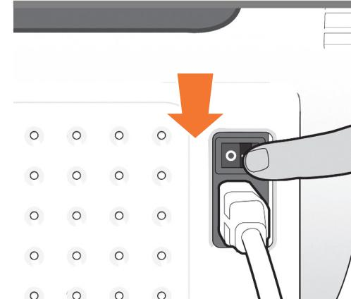
Switch on power to the product using the switch just above the power socket. Remove the plastic film covering the window and the plastic film covering the front panel (LCD display).
