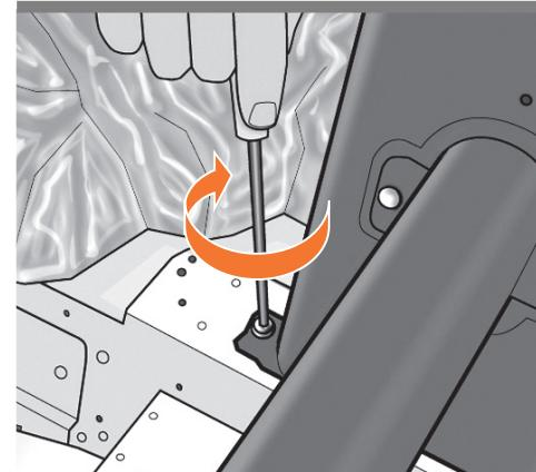
When the legs are correctly located on the product, attach them to the product using two screws for each leg. Check that you have used a total of twenty screws, and that all have been tightened. You should have two screws left over, which are spare.
