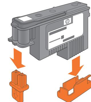
Unwrap each printhead and remove all orange parts.
