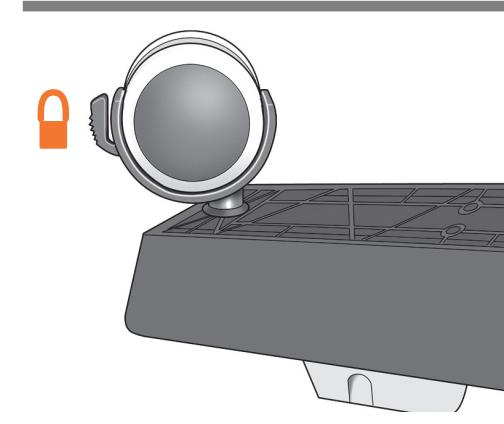
Check that the wheels on the stand are locked.
