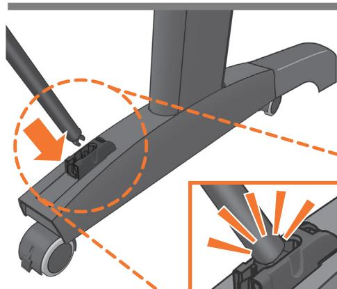
Fit the two short tubes to the product's feet, one on the front of each foot. Each tube should click into place.
