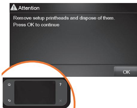
**EN** The setup printheads exist only to prevent the escape of ink during ink cartridge installation. The front panel now prompts you to remove the setup printheads and press the **OK** key when you have finished.
