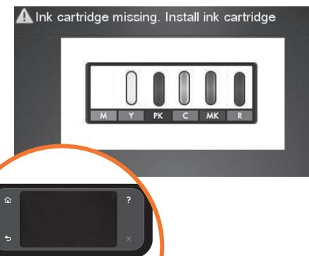
The product checks for the presence of ink cartridges. On finding none, it prompts you to install the ink cartridges.
