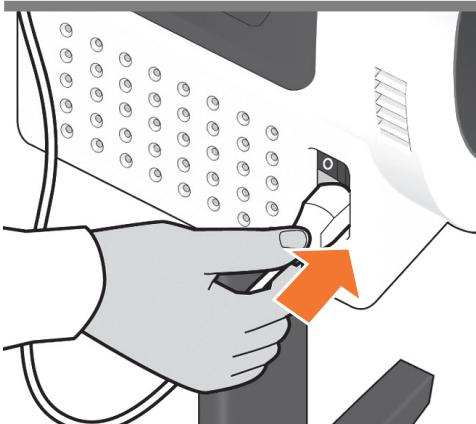
Connect the power cable to the product's power socket.
