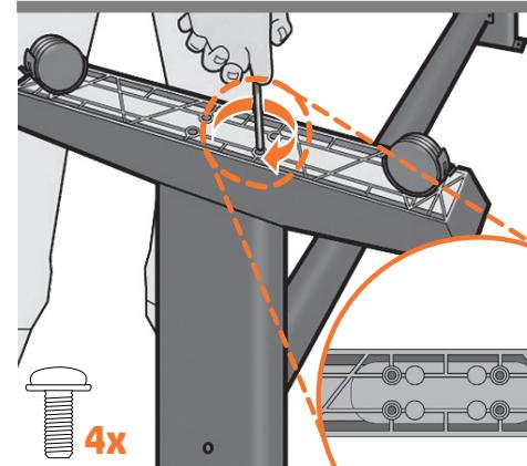
Attach a foot to each leg, using four screws in each foot. First fit all four screws loosely, then tighten them up.
