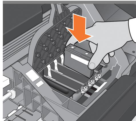
Insert the printheads one by one. Each printhead is marked with its own colors, and should be inserted only into the correct slot marked with the same colors. Insert the printheads with the blue handle towards you.
