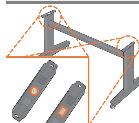
There is a round yellow button protruding from the top of one stand leg, and a square green button protruding from the top of the other leg. Each button fits into a hole in the product.
