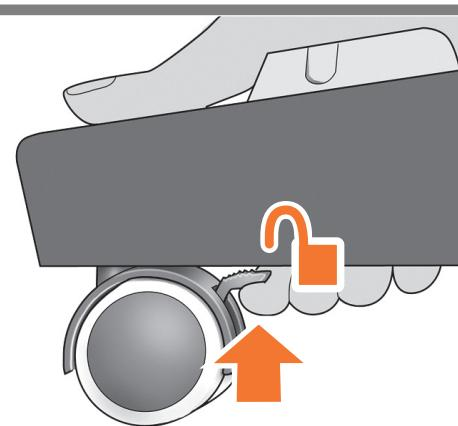
**EN** Unlock the brake lever on each of the four wheels by lifting the lever.
