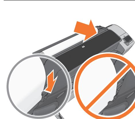
Feed the leading edge of the paper into the product until the product takes hold of it. Do not insert the roll paper into the cutsheet slot. **Note:** do not close the roll cover until the front panel notifies you.
