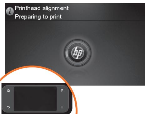
**EN** The product will proceed to align the printheads. This process involves printing, and therefore needs to use paper with a straight leading edge. **Note:** printhead alignment requires paper at least 24in (61cm) wide. Roll paper is recommended.
