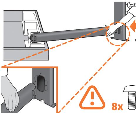
Support one end of the cross-brace on the stand box and attach a leg to the other end with two screws on the outside, then two on the inside of the leg. Don't fully tighten the screws yet. Attach the other leg following the same process. Now fully tighten the screws on the outside of the legs, followed by the screws on the inside.
