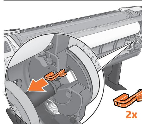
**Media load for lower roll** Go to the rear of the product, and remove the orange stoppers from each end of the spindle. **Note:** It is not necessary to install the 2nd roll to start using the product. If you prefer to install the 2nd roll later, please go directly to step 77.
