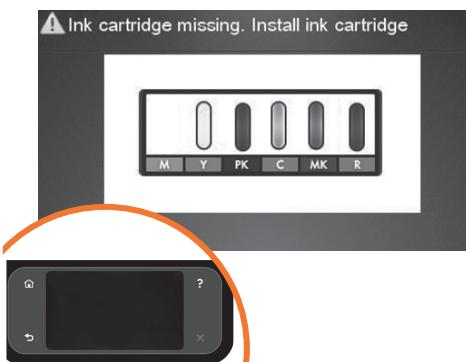
**EN** The product checks for the presence of ink cartridges. On finding none, it prompts you to install the ink cartridges.
