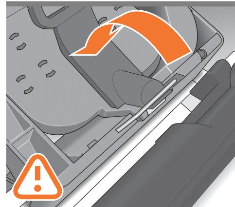
**Push the handle down on top of the printhead cover.**
