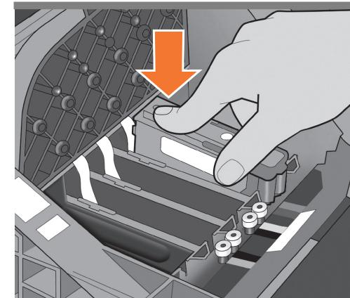
Push each printhead into the slot until it clicks into place. The front panel tells you whether the printhead has been inserted correctly.
