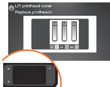
**EN** Press the OK key on the front panel when you have removed all of the setup printheads. The front panel then prompts you to install the new printheads.
