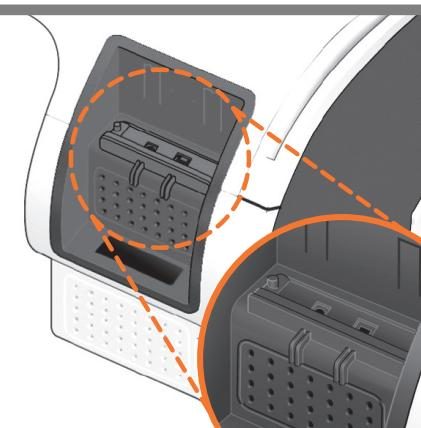
**EN** Connect the network cable and secure it with the clip provided, to prevent accidental unplugging.
