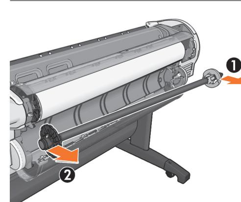
Remove the spindle by lifting out first the right-hand end, then the left.
