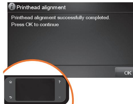
**EN** The front panel will display a series of messages showing the progress of the printhead alignment. There is no need to take any action until the alignment has finished, when you will see the message shown below. Press the OK key.
