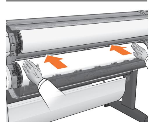
Feed the leading edge of the paper into the product until the product takes hold of it. Then move to the front of the product. **Note:** do not close the roll cover until the front panel notifies you. If the paper types of the two rolls differ, go to step 86 and calibrate the paper.
