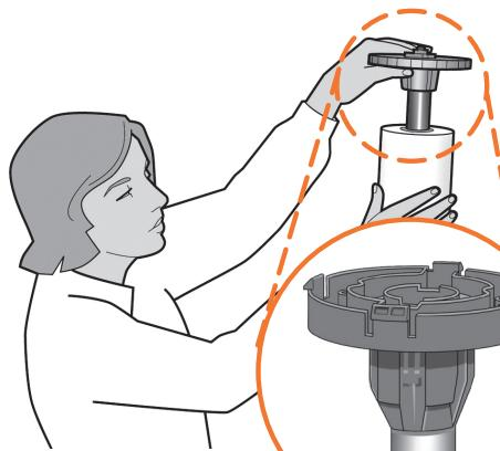
**EN** If the blue removable stop is on the spindle, remove it. Put the roll onto the spindle, making sure to put it on the right way round: the leading edge of the paper should go into the product from the top of the roll. Add the removable stop to the spindle to keep the roll in place.
