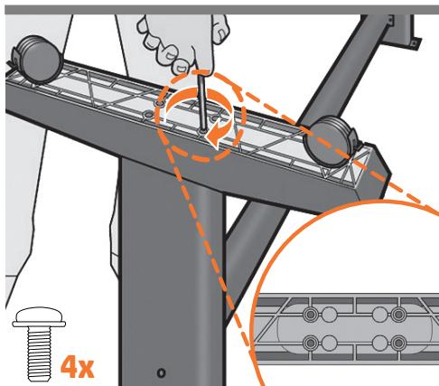
**EN** Attach a foot to each leg, using four screws in each foot. First fit all four screws loosely, then tighten them up.
