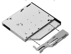
2. Slide the optical drive through the front bezel all the way into the bay so that it locks into place.
