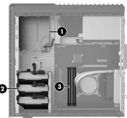
5. Disconnect the data and power cables from the rear of the drive (1), and then press the green release latch toward the center of the drive (2).
