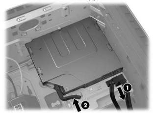
7. Remove the latch by pulling it away from the drive.
