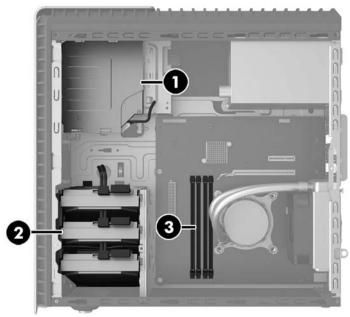
4. Disconnect the data and power cables from the rear of the hard drive (1). Pull the drive release lever (2), and then lift the drive up to remove it from the computer (3).
