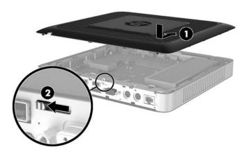
3. Insert the hooks on the right side of the rear I/O panel (1) into the right side of the back of the chassis, rotate the left side (2) to the chassis, and then press it to the chassis until it locks in place.
