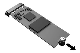
11. Pull the screw kit off of the storage module and attach it to the replacement storage module.
