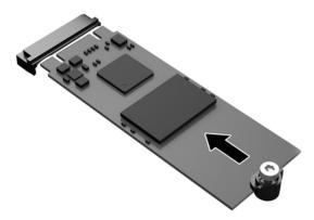
NOTE: A storage module can be installed in only one way.
