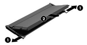
10. Slide the new memory module (1) into the socket at approximately a 30° angle, and then press the memory module down (2) so that the latches lock it in place.
