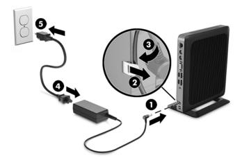
CAUTION: Failure to secure the power cable with the retention hook may result in the AC power cord becoming disconnected, causing loss of data.
