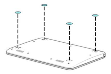
To install the rubber feet, remove the protective backing from the rubber feet and install them in the locations indicated in the above illustration.
