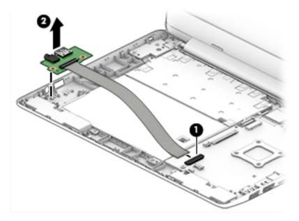
Reverse this procedure to install the connector board and cable.
