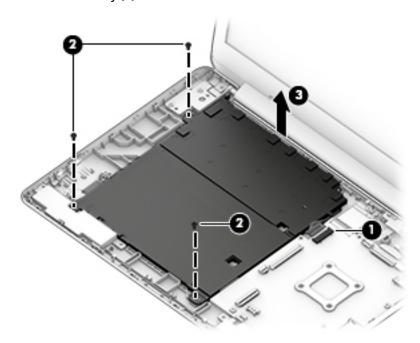
Reverse this procedure to install the battery.
