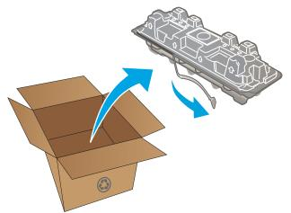
5. Remove the new toner cartridge from the opened packaging shell. Place the used toner cartridge in the shell for recycling.
