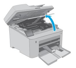
3. Remove the used toner cartridge from the printer.
