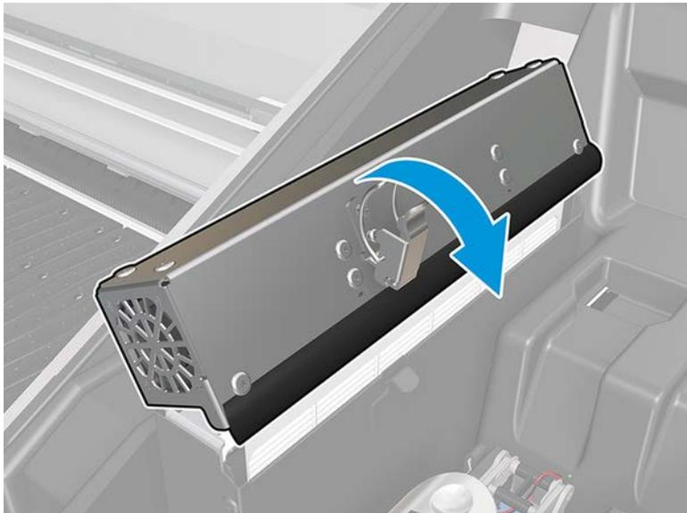
6. Extract the frame from the aerosol container and remove the filter from the frame.
