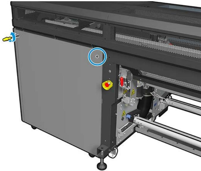
4. Remove the rear right panel assembly and locate the first Dryer PCA fan filter.
