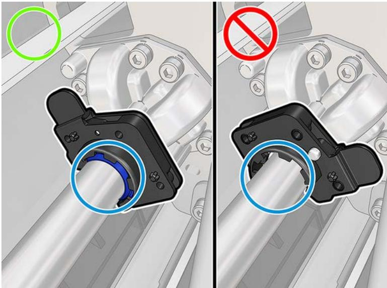
5. Insert the oiling felts into each rail and slide towards the carriage. Notice the cross shaped features in the oiler felt housing shown below have to go into the holes provided in the carriage. Also, for the rear oiler felt notice two pins in the carriage have to pass through holes in the oiler felt housing.
