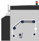
The substrate goes from the input spindle (1) over the main roller (2), over the platen (3), over the front diverters (4) and then to the output spindle (5).
