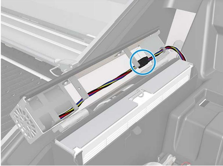
10. Remove the main cable harness from the cover slot.
