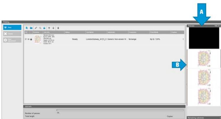
**NOTE:** When tiling optimized substrate is loaded, the specific workflow changes and beginning of job preparation plot and sideways color bars are automatically introduced. Workflow for non-optimized substrates is not affected.
