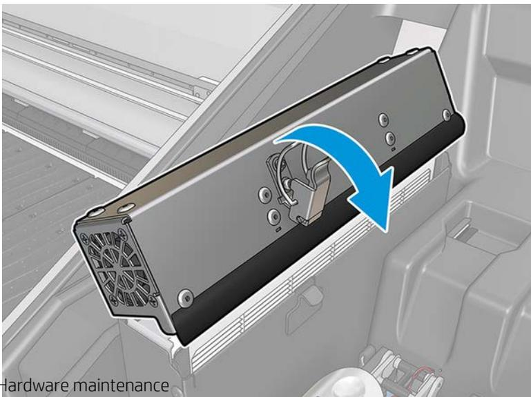
8. Remove the two screws that attach the cover, and remove the cover.
