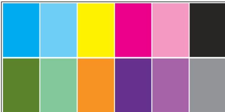
When facing banding issues, print the Image Quality Inspection Plot from the **Printer** menu: go to **Printer > IQ Inspection > Add New Job**. This will add a job to the print queue. To print it, edit the details of the job to select the substrate and print mode you want to check. Once the plot has printed, start the troubleshooting process. See
