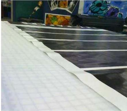
1. Check that the substrate type you have loaded corresponds to the substrate type selected in the Internal Print Server and in your software.
