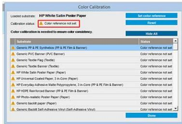
**NOTE:** After creation, a CLC is required to create the reference for future color calibration. A warning window appears straight after substrate creation. You can create an ICC profile from the RIP and manage the substrate as normal from this point on.
