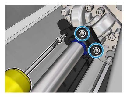
2. Remove and guard the metal part covering the rear oiling felt.
