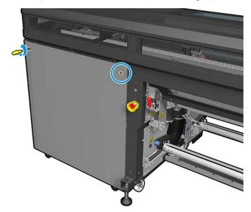
Remove the rear right panel assembly and locate the first Dryer PCA fan filter.
