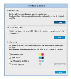
2. Press the **Check** button to perform routine cleaning automatically.
