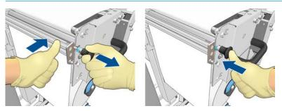
13. Grip the handle and push the whole printhead cleaning roll assembly back into the printer. Ensure that you push it as far as it will go.
