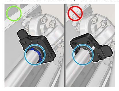
5. Insert the oiling felts into each rail and slide towards the carriage. Notice the cross shaped features in the oiler felt housing shown below have to go into the holes provided in the carriage. Also, for the rear oiler felt notice two pins in the carriage have to pass through holes in the oiler felt housing.
