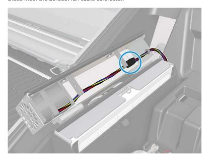
10. Remove the main cable harness from the cover slot.
