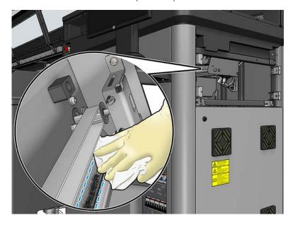
Lubricate the 2 rods with a few drops of oil.
