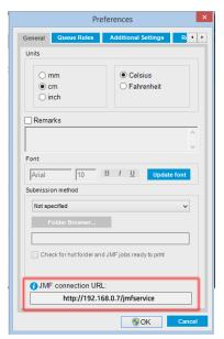
If there are problems using the printer's hostname, switch to the printer's IP using the HP Latex 1500 System Configuration Tool. For more details refer to the Service Manual or talk to your network administrator to solve hostname resolution.
