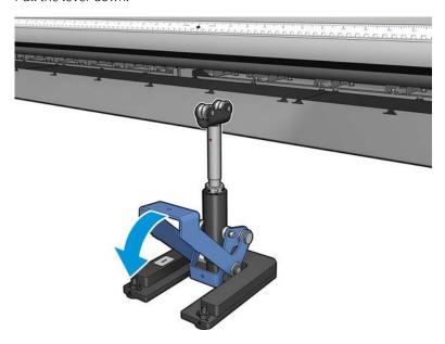
Adjust the height of the support by turning it counterclockwise. The bearings at the top of the dual-roll center support must touch the spindle.
