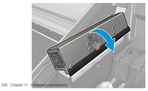
8. Remove the two screws that attach the cover, and remove the cover.
