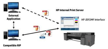
If you are using CALDERA 10.2 RIP, then the MIS can communicate using the Caldera Nexio module. **Caldera Nexio** is a tool that connects the Caldera RIP and other third-party software using standard JDF/JMF protocols, making it possible to produce automatic sequences of actions that speed up production and advanced reports to improve operations. Please, contact CALDERA for further information.
