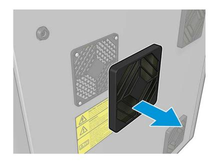
2. Take the fan filter and clean by blowing it with the air gun. Be careful to locate it back correctly: it must cover the fan's square surface.
