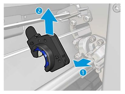
Take the two clean left oiling felts from the printer maintenance kit and install them. Make sure that once installed the blue plastic part in the oiler felt has to be outwards (not inwards).
