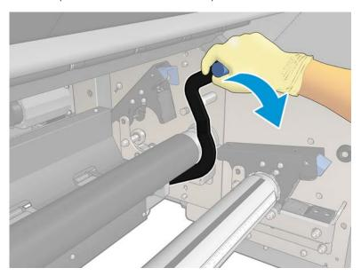
3. Clean the pinchwheels carefully with a cloth dampened with water (for persistent dirt you may use isopropyl alcohol, but do not use petroleum-based cleaning liquids).
