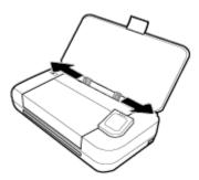
3. Insert the paper print-side up and slide the paper-width guides till they fit snugly against the sides of the paper.
