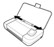
Insert the paper print-side up and slide the paper-width guides till they fit snugly against the sides of the paper.
