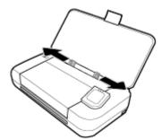
3. Insert the envelope print-side up and the long-edge flap on the left or the short-edge flap at the top.
