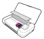
**3.** Open the cartridge latch as shown and gently remove the cartridge from its slot.
