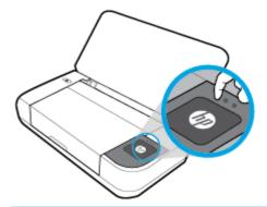
**NOTE:** Return the printer control panel to its original position by pushing down the top side until it clicks into place.
