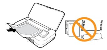
Slide the paper-width guides inward until they stop at the left and right edges of the paper.
