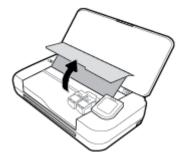
Remove all visible paper by moving the cartridges around from one side to the other.
