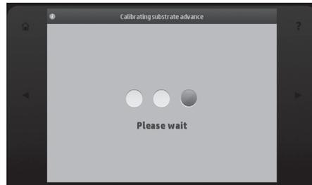
The printer automatically performs substrate advance calibration and printhead alignment. Please do not stop those processes to ensure successful printhead alignment.
