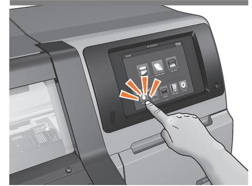
**HP Latex 570 Printer only:** Press OK on the front panel.
