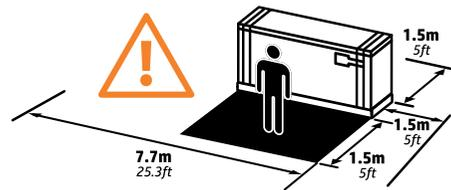
**EN** The space required for assembly is 1.5 m (5 ft) front and rear, and 7.7 m (25.3 ft) at the side.
