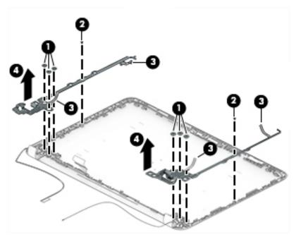
5. To remove the wireless cable and antenna (1), release the cable from the clips built into the display enclosure (2), and then remove the cable and antenna.
