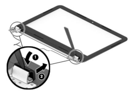
c. At the seam in the bottom of the display, use a plastic, non-marking tool (1) to separate the bezel(2) from the display enclosure.
