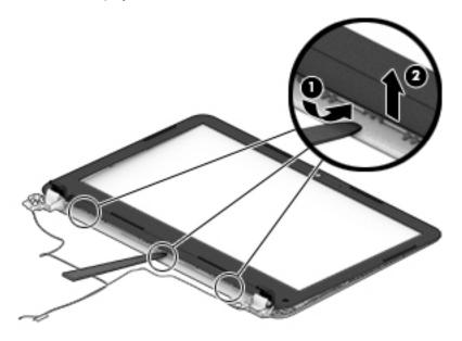
**d.** Lift the left (1), top (2), and the right sides (3) of the bezel to loosen it from the display. Lift the bezel off the display (4).
