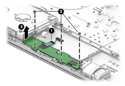
Reverse this procedure to install the TouchPad button board and cables.
