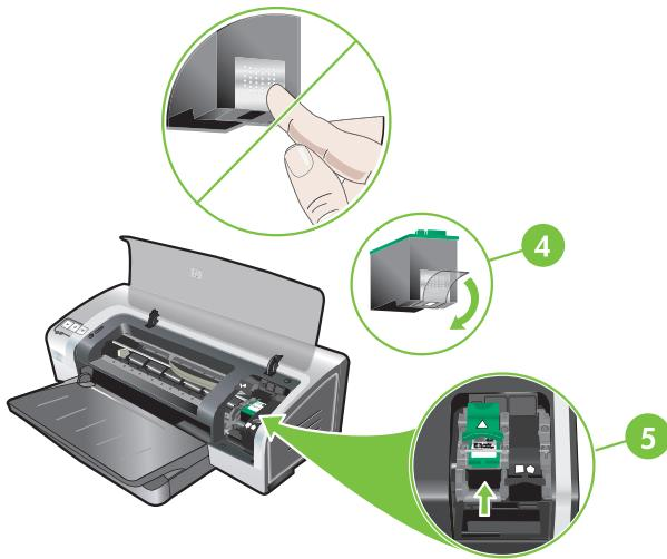
4) Remove the tri-color print cartridge from its package, and then remove the clear nozzle protective tape by pulling on the pink pull-tab. **Caution:** Do not touch the ink nozzles or copper contacts, and do not remove the copper contacts. 5) Insert the tri-color print cartridge into the left cradle.
