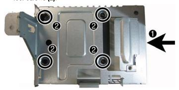
3. Insert the cable into the clip on the drive cage (1), and then replace the screw (2).
