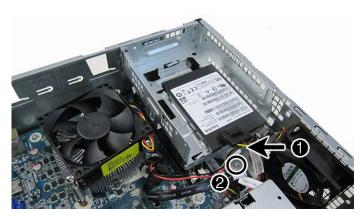
5. Connect the data and power cables to the back of the hard drive. Note that a 3.5-inch drive is shown.
