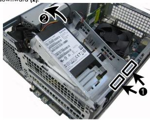
4. To install a 3.5 inch hard drive: Orient the hard drive to match the orientation of the old hard drive-that is, which side is up and the position of the connector. Insert the hard drive into the drive cage (1), and then replace the four screws (2).
