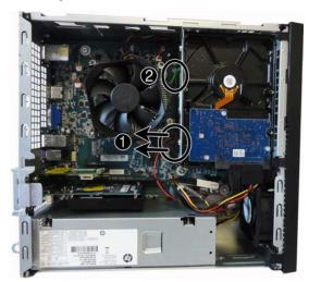
8. Disconnect the power and data cables from the back of the hard drive. Note that a 3.5-inch drive is shown.
