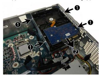
10. To remove a 2.5-inch hard drive you must remove the hard drive cage. Remove the screw that secures the hard drive cage to the computer (1), remove the cable from the clip in the cage (2), and then rotate the cage up and remove it from the computer (3).
