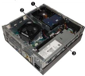
5. Remove the fan duct to access the cables connected to the rear of the optical drive. Pull the tabs away from each other (1), and then lift the duct off the fan sink (2).
