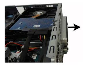
4. To remove the front bezel, pull the three tabs upward (1), and then rotate the bezel off the computer (2).
