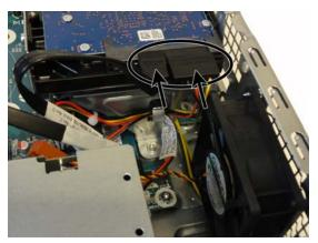
2. To replace the hard drive cage, insert the tabs at the top of the cage into the slots in the side of the computer (1), and then rotate the drive cage downward (2).
