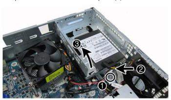
11. To remove the 2.5-inch hard drive from the drive cage, remove the four Phillips screws from the bottom of the cage (1), and then slide the drive out of the drive cage (2).
