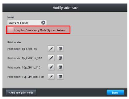
NOTE: The name of this feature for HP Latex 310 and 330 units is just "Long Run Consistency Mode," without the last informative description ("System Preheat").
