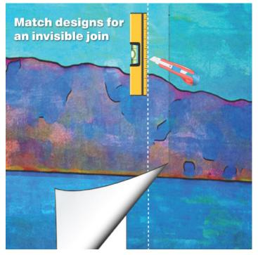
Double-cutting is a technique that is used to obtain perfectly fitted seams. It is done by overlapping one panel of wallpaper over the other until the image or patterns are perfectly matched. Then a sharp blade is used to cut through both layers. The excess edges are then removed.
