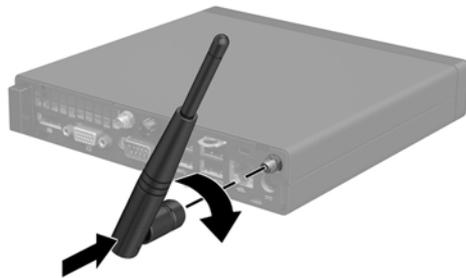
10. Connect the external antenna cables to the WLAN module.
