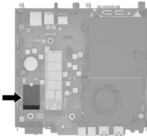
6. Disconnect both antenna cables from the WLAN module.
