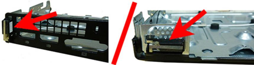
15. Remove the front antenna from the inside of the computer by pressing the tab to disengage the transceiver and removing the transceiver (arrow in following image points to the tabs on the inside of the computer).
