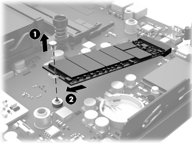
8. Insert the new SSD into the socket on the system board.
