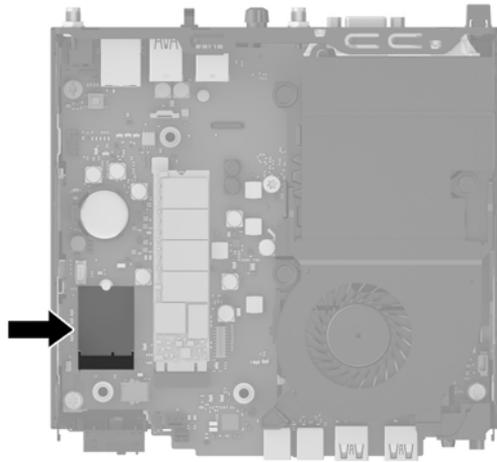
6. Disconnect the internal antennae from the WLAN module.
