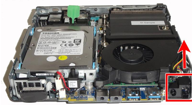
To install the power switch/light cover, reverse the removal procedure.
