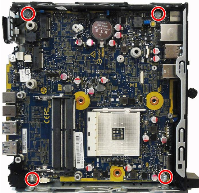
To install the system board, reverse the removal procedures.
