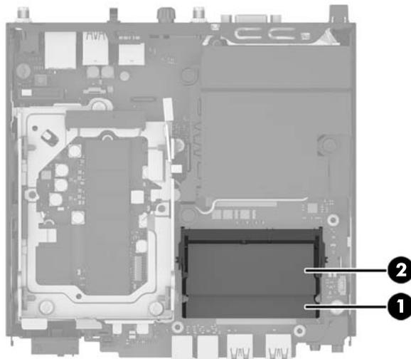
9. To remove a memory module, press outward on the two latches on each side of the memory module (1), and then pull the memory module (2) out of the slot.
