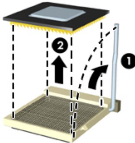
Reverse the removal procedure to install a new processor.
