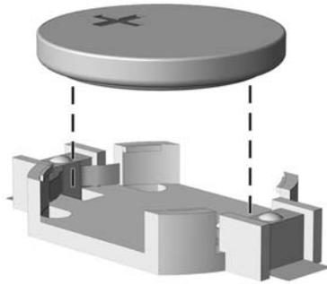
7. Slide the replacement battery into position, positive side up. The battery holder automatically secures the battery in the proper position.
