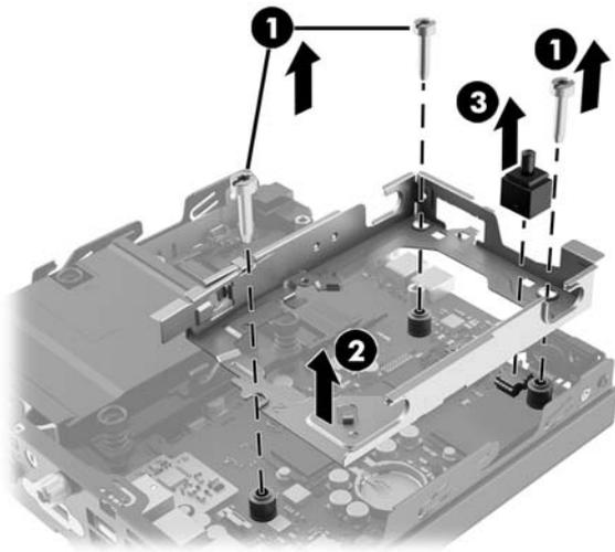
To install the drive cage, reverse the removal procedure.
