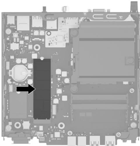
6. Remove the screw **(1)** securing the SSD to the system board.
