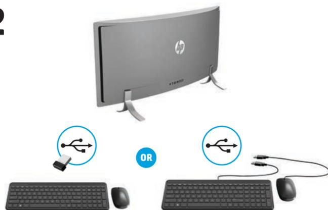
**NOTE:** Depending on the model number of your product, the USB transceiver is either preinstalled in your product or located inside the mouse box. For setup instructions for the mouse, see the outside of the mouse box. For setup instructions for the keyboard, see the outside of the keyboard box.
