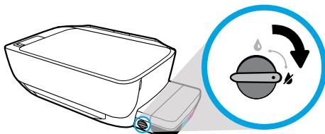
You must lock valve (horizontal position) before moving or tilting printer, so ink will not leak.
