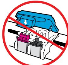
After printheads have been primed with ink, you must not open blue carriage latch. Opening latch can cause permanent damage to printheads.
