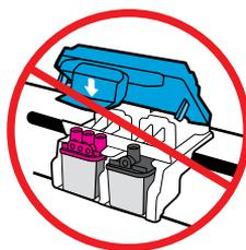
After printheads have been primed with ink, you must not open blue carriage latch. Opening latch can cause permanent damage to printheads.
