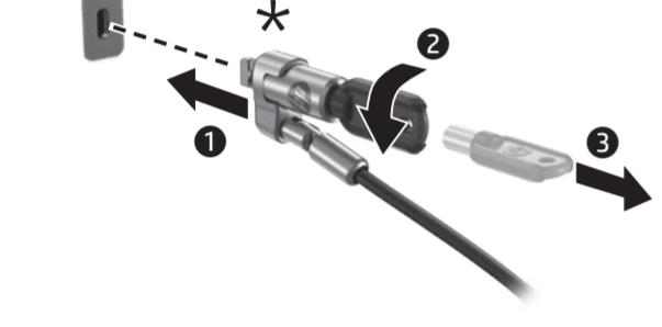
\*Security cable not included. Install the security cable in the bottom module to lock all modules together.
