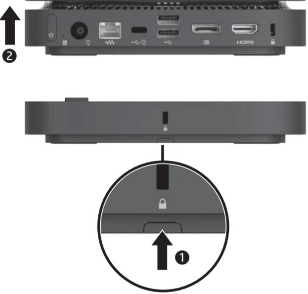
Modules must be removed one at a time, starting from the bottom. For each module, press the release latch ①, and then remove the module ②.
