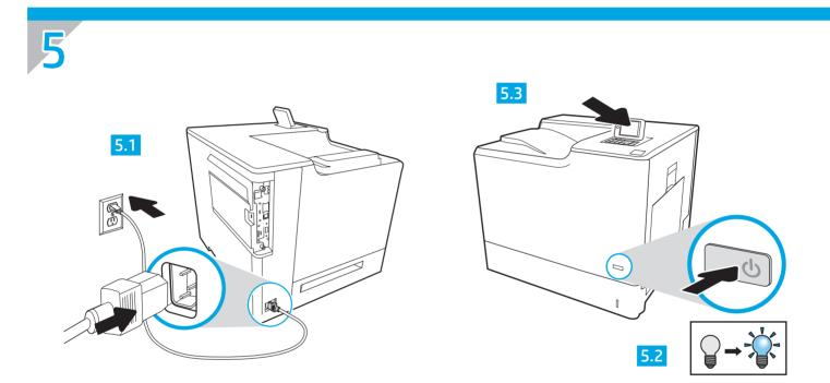
EN 5.1 Connect the power cable between the printer and a grounded AC outlet. 5.2 Turn on the printer. 5.3 On the Initial Setup screen, set the language, the location, the date/time format, and other features.
