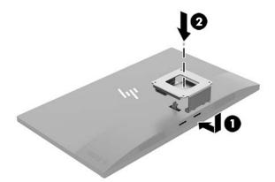
4. To attach the monitor to a swing arm or other mounting device, insert four mounting screws through the holes on the mounting device and into the screw holes on the VESA bracket.
