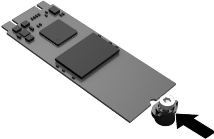
12. Slide the new flash storage module into the M.2 socket on the system board and press the module connectors firmly into the socket.
