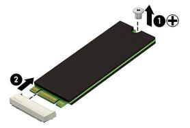
Reverse this procedure to install the solid-state drive.
