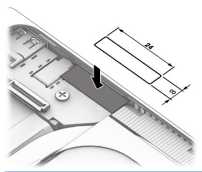
**IMPORTANT:** The acetate tape is not spared and must be obtained locally.
