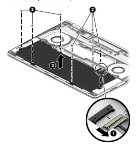
Reverse this procedure to install the battery.
