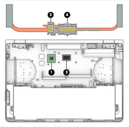
Reverse this procedure to install the heat sink.
