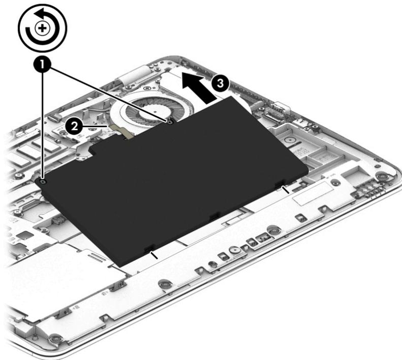
Reverse the removal procedures to install the battery.
