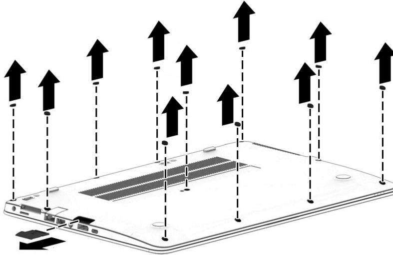
3. Remove the 11 Phillips M2.5x5.0 screws (1) - (11) and the Phillips M2.0x7.0 screw (12) in the order shown in the following image.
