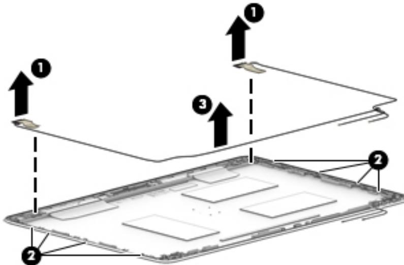
15. If it is necessary to replace the WWAN antenna cables, peel the transceivers from the top of the display enclosure (1), remove the antenna cables from the on the sides of the display enclosure (2), and then remove the antenna cables (3).
