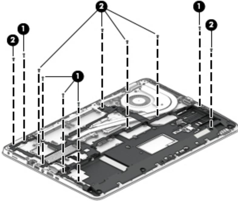
2. Remove the 5 broadhead Phillips M2.5x2.5 screws that secure the internal base plate to the computer **(3)**.
