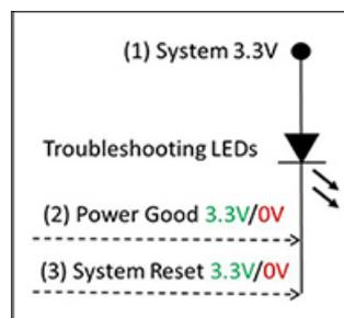
These lights should be visible after removing the service door or bottom cover. Consult with support for platform-specific locations of the lights.
