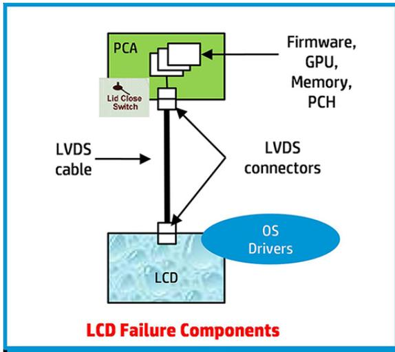
**NOTE:** The lid close switch is a Hall-effect sensor located in the top cover. When the display is closed, the sensor acts like a switch. A notebook can force a video output to an external monitor, or go to hibernation or standby mode through power management. If the display screen does not light up when the display is open, the lid close switch (Hall-effect sensor) could be faulty.
