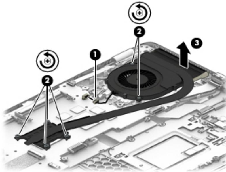
4. UMA graphics models: The thermal material must be thoroughly cleaned from the surfaces of the heat sink and the system board components each time the heat sink is removed. Replacement thermal material is included with the heat sink, processor, and system board spare part kits.
