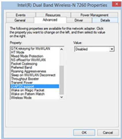
point. If disabling U-APSD improves the throughput issue, check with the access point provider for updated firmware that resolves the issue.
