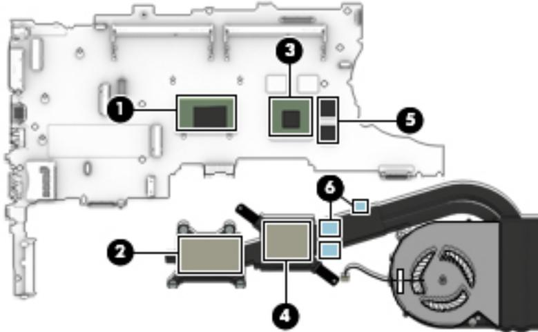
3. UMA graphics models: Loosen the six captive screws on the fan and heat sink following the sequence stamped on the fan and heat sink (1), disconnect the fan cable from the system board (2), and then remove the heat sink/fan assembly from the system board (3).
