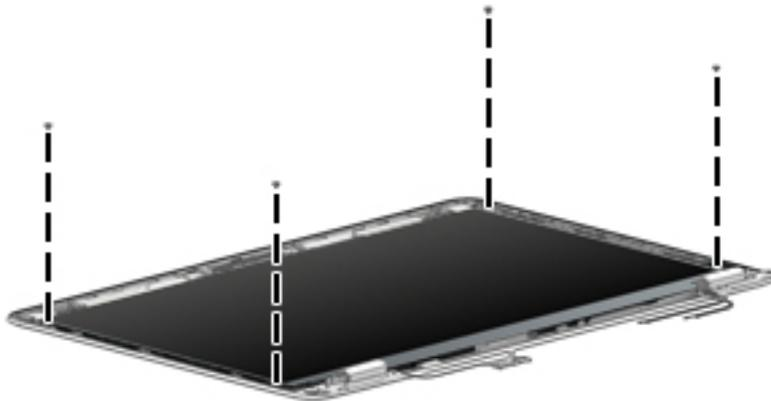
8. Rotate the display panel over onto the keyboard **(1)**
