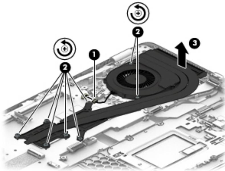
2. Discrete graphics models: The thermal material must be thoroughly cleaned from the surfaces of the heat sink and the system board components each time the heat sink is removed. Replacement thermal material is included with the heat sink, processor, and system board spare part kits.
