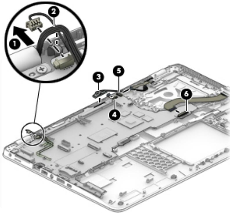
5. Remove the 2 Phillips M2.5×5.0 screws (1) that secure the system board to the computer.
