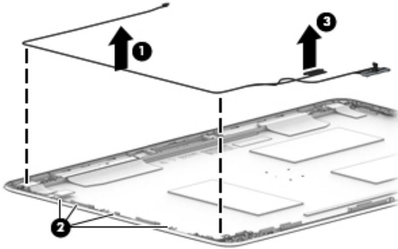
14. If it is necessary to replace the WLAN antenna cables, peel the transceivers from the top of the display enclosure (1), remove the antenna cables from the routing path on the sides of the display enclosure (2), and then remove the antenna cables (3).
