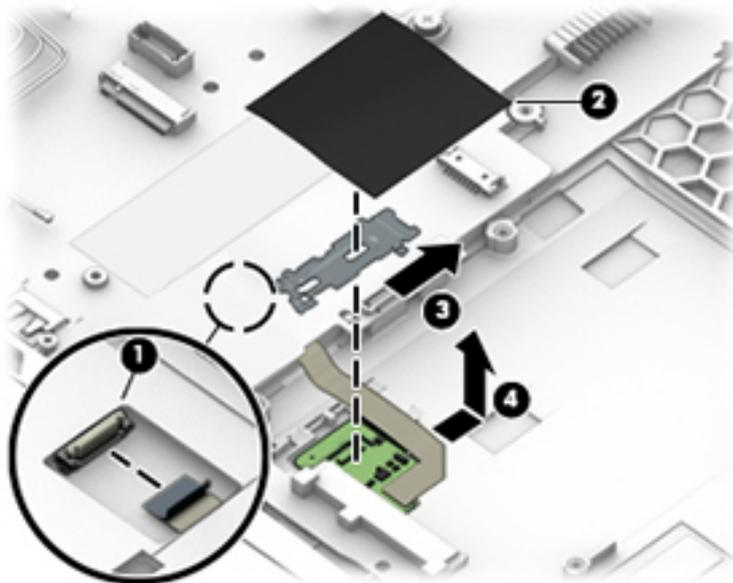
Reverse this procedure to install the fingerprint reader assembly.
