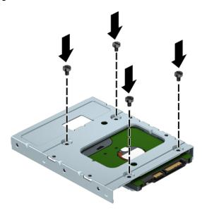
Install four 6-32 silver-and-blue mounting screws in the adapter bracket (two on each side of the bracket).
