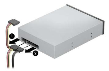
**5.** Push the green drivelock mechanism towards the optical drive **(1)**, and then slide the drive from the drive bay **(2)**.
