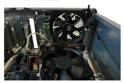
To install the fan assembly, reverse the removal procedure. Be sure to orient the air flow out of the chassis.
