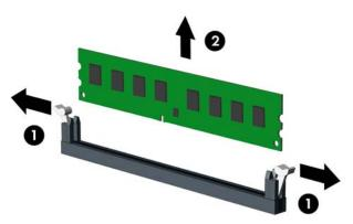
**4.** To install a memory module, open both latches of the memory module socket **(1)**, and insert the memory module into the socket **(2)**.
