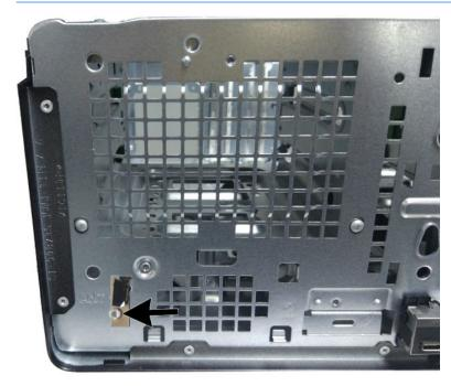
5. From the inside, rear of the computer, press the tab that secures the antenna cover to the computer.
