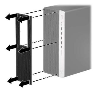
Use a soft brush or cloth to clean dust from the filter. If heavily soiled, rinse the filter clean with water.
