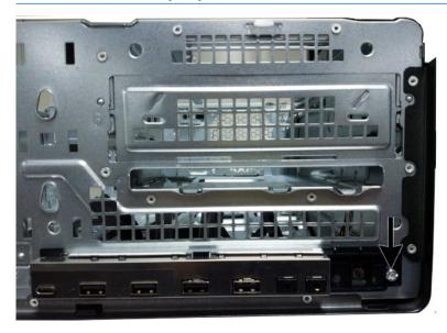
7. Rotate the right side of the assembly away from the computer, and then pull the assembly out of the front of the chassis while threading the cables through the hole in the front of the chassis.
