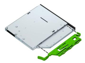
5. Slide the optical drive through the front bezel all the way into the bay (1) so that the latch on the rear of the drive locks into place (2).
