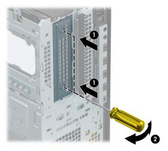
6. Slide the drive into the drive bay, making sure to align the mounting screws with the mounting slots, until the drive snaps into place.
