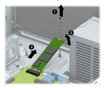
5. To install an M.2 SSD card, slide the pins on the card into the system board connector while holding the card at approximately a 30° angle (1). Press the other end of the card down (2), and then secure the card with the screw (3).
