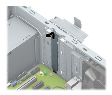
The other two slot covers must be removed with a screwdriver. Insert a flat-bladed screwdriver into the slots on the rear of the slot cover (1) and rock the slot cover back and forth (2) to break it free from the chassis.
