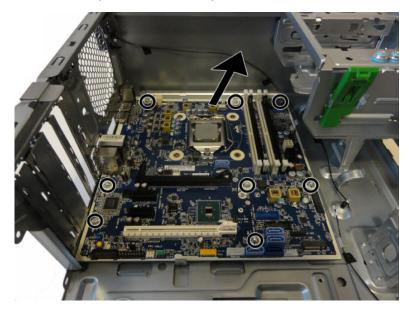
When reinstalling the system board, first insert the I/O panel back into the slots in the rear of the chassis, and then align the board with the chassis screw holes.
