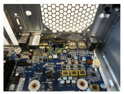
To install the option board, reverse the removal procedures.
