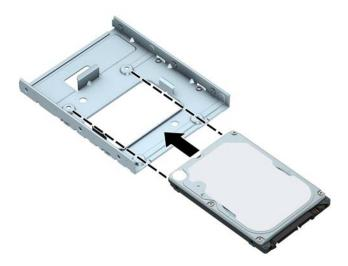
Secure the drive to the bay adapter bracket by installing four black M3 adapter bracket screws through the underside of the bracket and into the drive.
