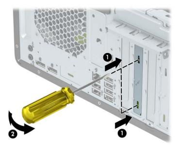
**b.** If you are removing a PCI Express x1 card, hold the card at each end and carefully rock it back and forth until the connectors pull free from the socket. Lift the card straight up **(1)**, and then away from the inside of the chassis **(2)** to remove it. Be sure not to scrape the card against other components.
