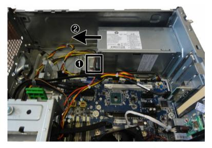
To install the power supply, reverse the removal procedure.
