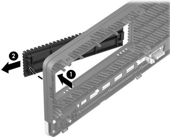
To remove a slim optical drive bezel blank, press inward on the tab on the right side of the blank **(1)**, and then rotate the blank away from the front bezel **(2)** and slide the left side of the blank out of the slot on the front bezel **(3)**.
