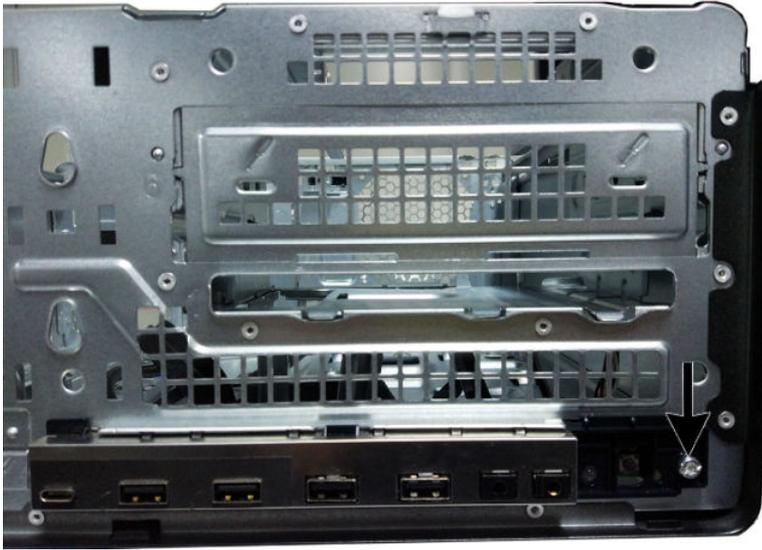
7. Rotate the right side of the assembly away from the computer, and then pull the assembly out of the front of the chassis while threading the cables through the hole in the front of the chassis.
