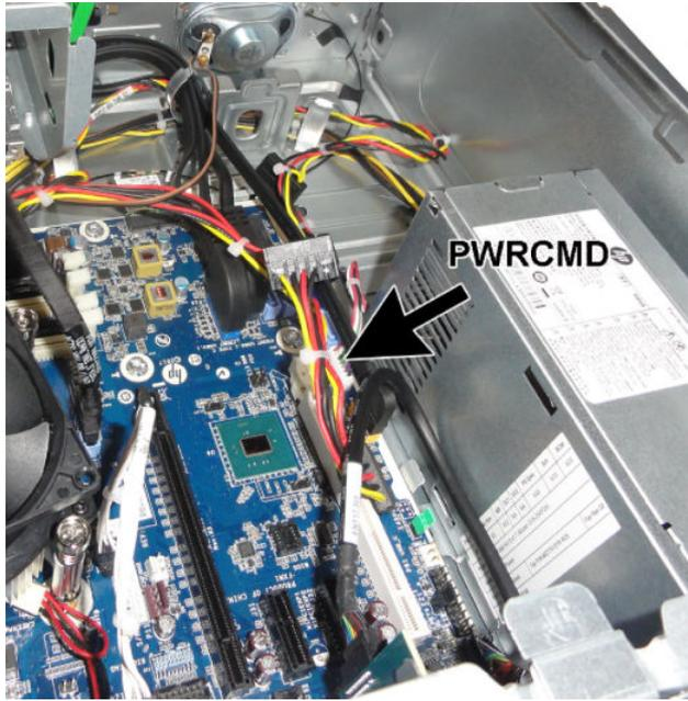
7. Disconnect the power supply cables from the following system board connectors:
