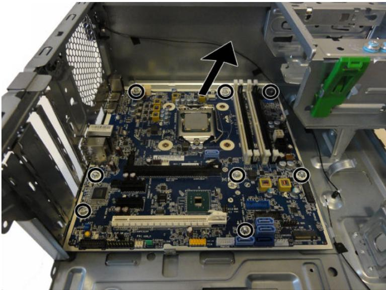
When reinstalling the system board, first insert the I/O panel back into the slots in the rear of the chassis, and then align the board with the chassis screw holes.
