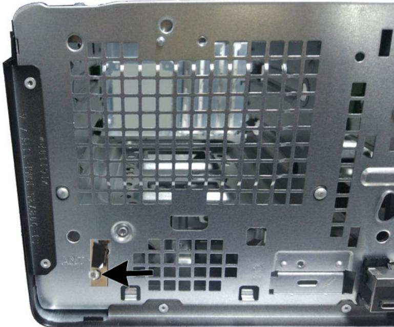
5. From the inside, rear of the computer, press the tab that secures the antenna cover to the computer.
