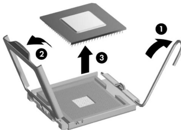
Reverse the removal procedure to install a new processor.
