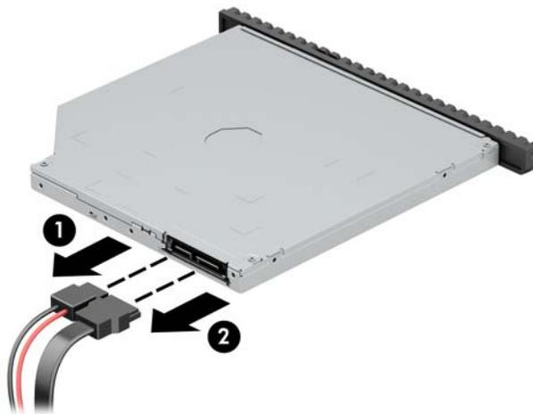
4. Push the green release latch on the right rear side of the drive toward the center of the drive **(1)**, and then slide the drive forward and out of the bay **(2)**.
