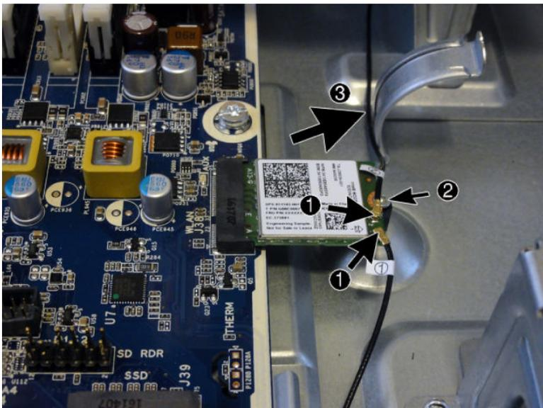
Reverse this procedure to install the WLAN module.
