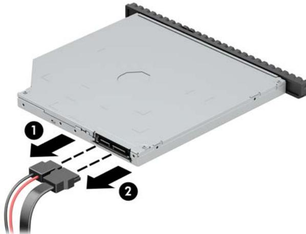
5. Push the green release latch on the right rear side of the drive toward the center of the drive **(1)**, and then slide the drive forward and out of the bay **(2)**.
