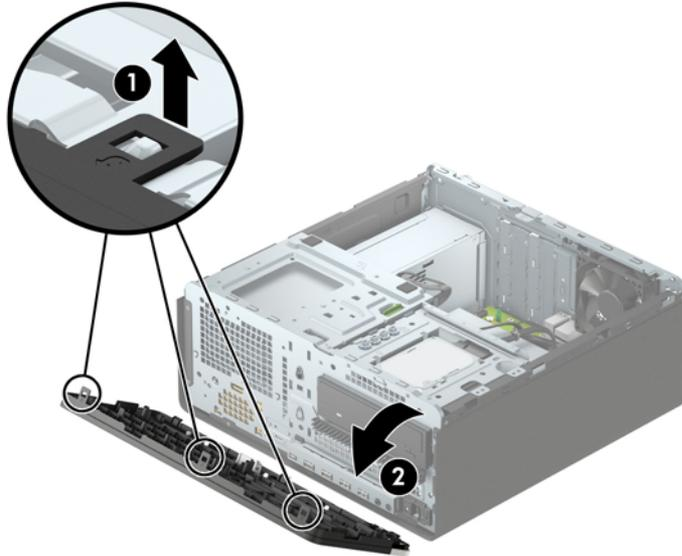
To replace the front bezel, reverse the disassembly procedures.
