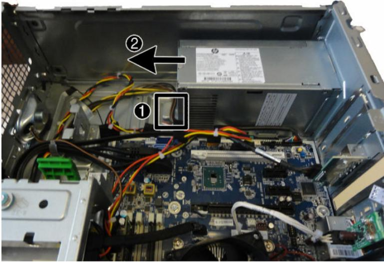
To install the power supply, reverse the removal procedure.
