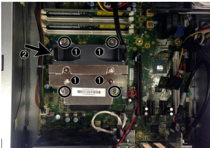
5. Lift the heat sink from atop the processor.
