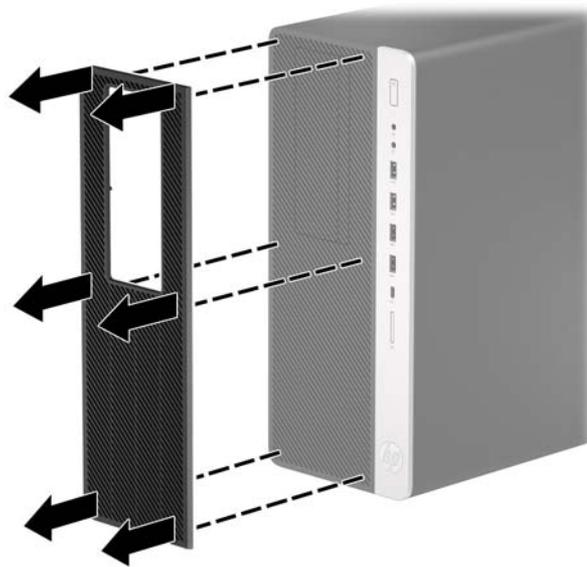
3. Use a soft brush or cloth to clean dust from the filter. If heavily soiled, rinse the filter clean with water.
