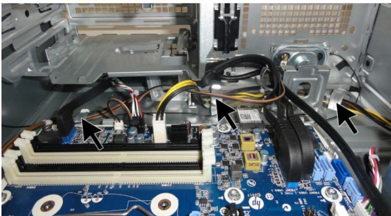
6. Disconnect the power supply cables from the following system board connector:
