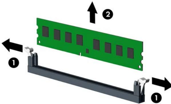
4. To install a memory module, open both latches of the memory module socket **(1)**, and insert the memory module into the socket **(2)**.
