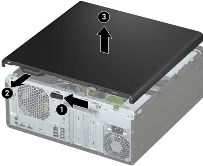
To replace the access panel, reverse the disassembly procedures.
