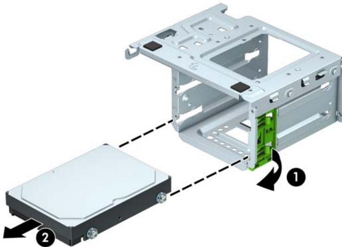
5. Remove the four mounting screws (two on each side) from the old drive. You will need these screws if you install a new drive.
