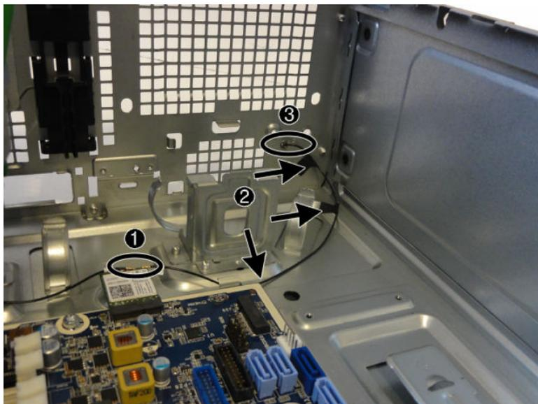
Reverse the removal procedure to install the WLAN antennas and transceivers.
