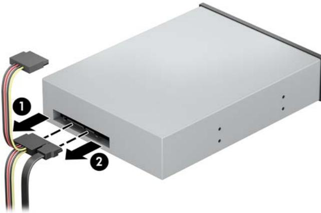
5. Push the green drivelock mechanism towards the optical drive **(1)**, and then slide the drive from the drive bay **(2)**.
