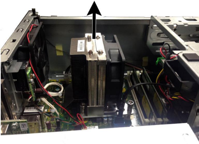
When reinstalling the fan sink, make sure that its bottom has been cleaned with an alcohol wipe and fresh thermal grease has been applied to the top of the processor.
