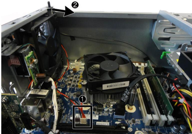
To install the hood sensor, reverse the removal procedure.
