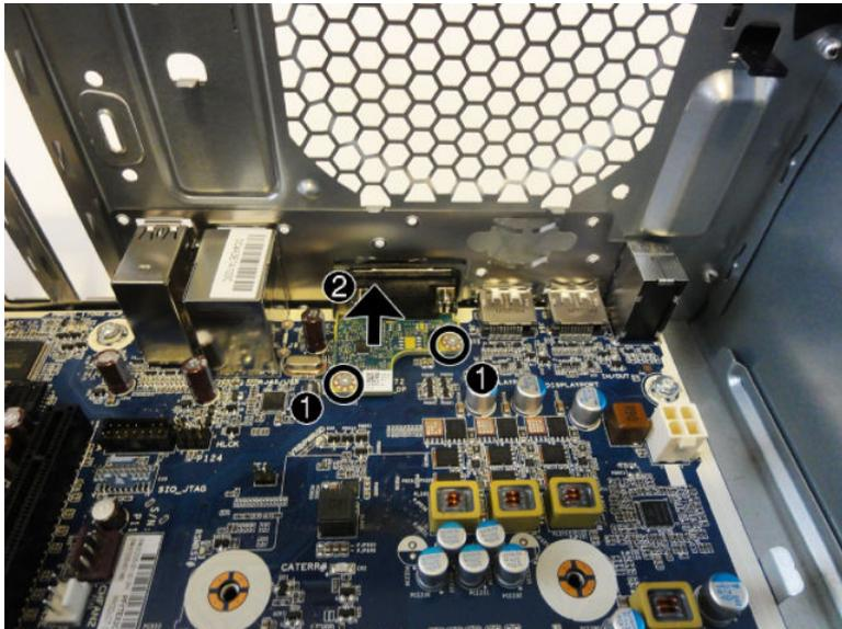
To install the option board, reverse the removal procedures.
