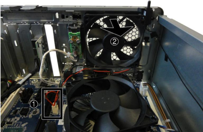
To install the fan assembly, reverse the removal procedure. Be sure to orient the air flow out of the chassis.
