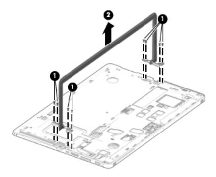
To remove the hinges, remove the screws (1) securing the hinges to the kickstand, and then remove the brackets (2).
