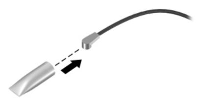
Reverse this procedure to replace the WWAN or GPS module (select products only).
