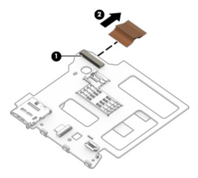
Reverse this procedure to replace the smart card reader board and bracket.
