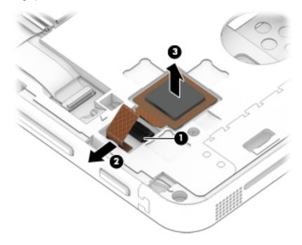
Reverse this procedure to replace the fingerprint reader board.
