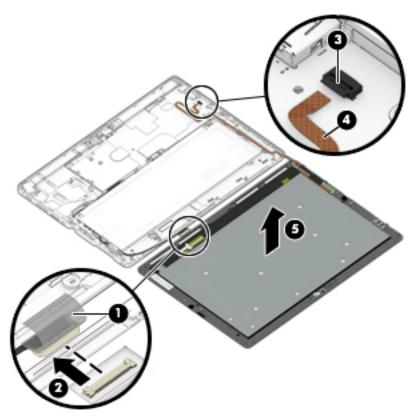
Reverse this procedure to replace the display panel.
