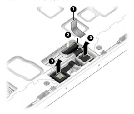
Reverse this procedure to replace the rear webcam.
