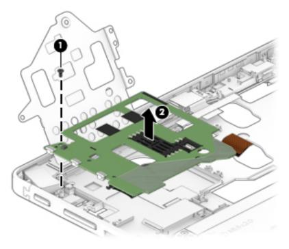
6. To remove the ribbon cable, turn over the smart card reader board, open the ZIF connector (1), and then remove the cable (2).
