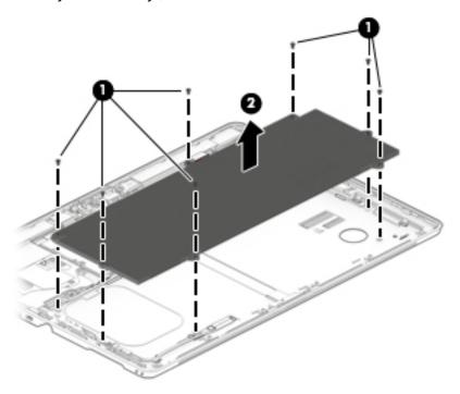
Reverse this procedure to replace the battery.
