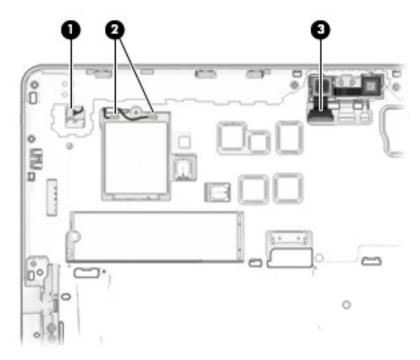
5. Release the following cables from the system board:
