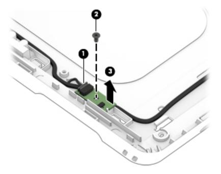
Reverse this procedure to replace the Hall effects sensor board.
