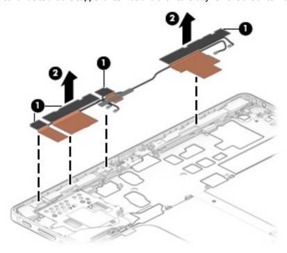
Reverse this procedure to replace the antennas.
