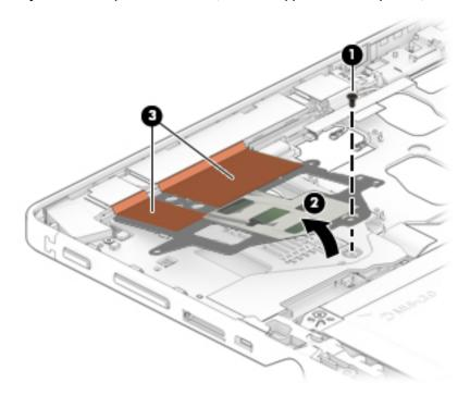
4. Remove the Phillips M1.6x3 screw (1) securing the smart card reader board.
