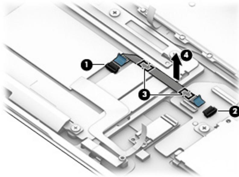
Reverse this procedure to install the TouchPad cable.
