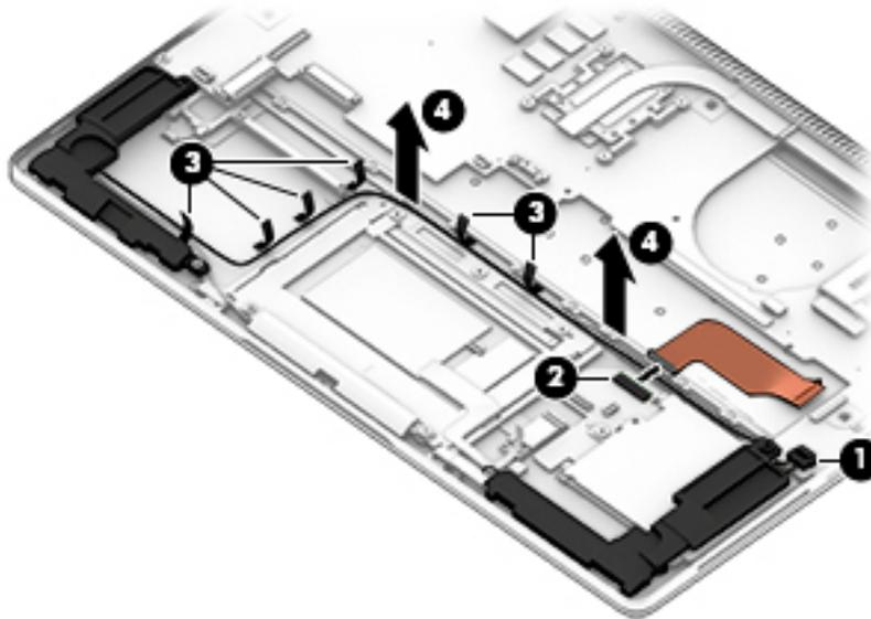
5. Remove the two Phillips PM2.0×2.4 screws **(1)** that secure the speakers to the keyboard/top cover.
