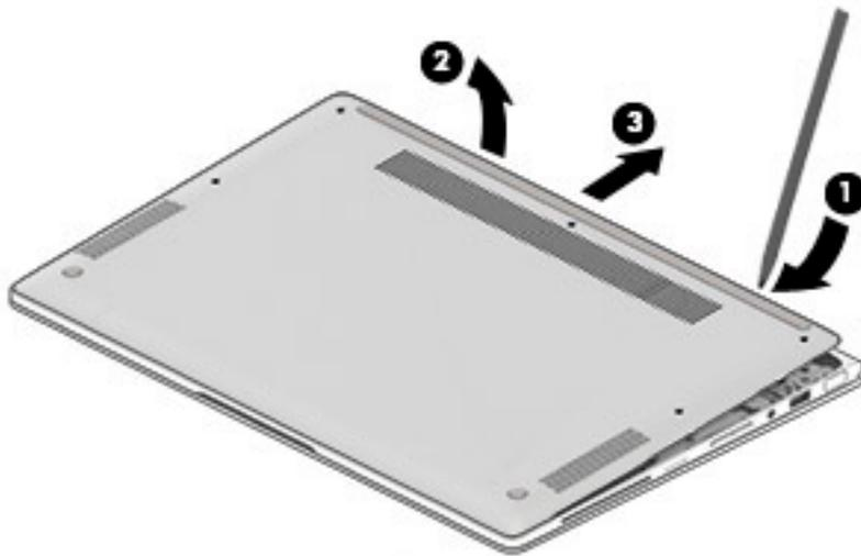
Reverse this procedure to install the bottom cover.
