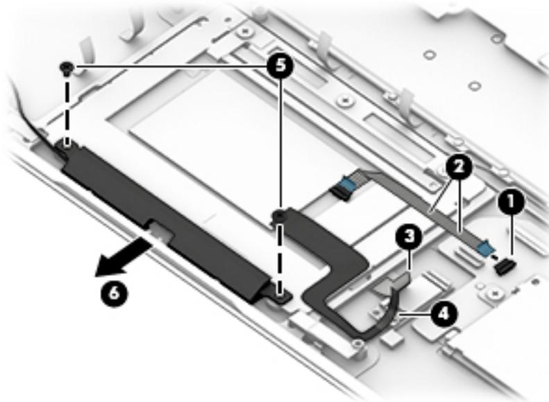
7. Remove the four Phillips PM2.0×2.4 screws **(1)** that secure the TouchPad to the keyboard/top cover.
