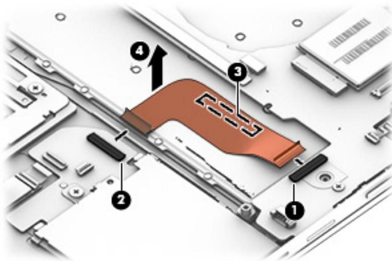
Reverse this procedure to install the card reader board cable.
