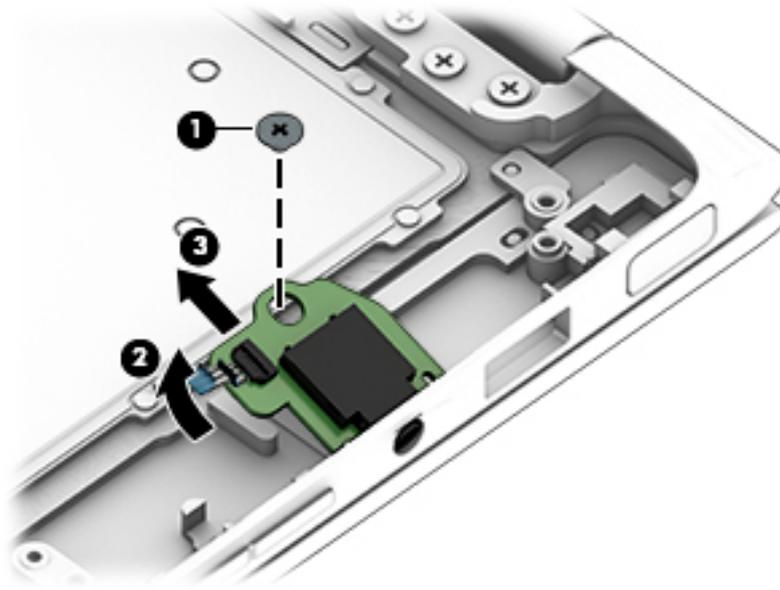
Reverse this procedure to install the audio jack board.
