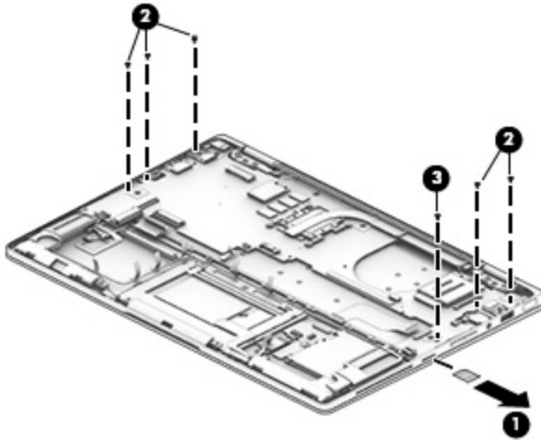
4. Lift the front edge of the system board **(1)** until it rests at an angle.
