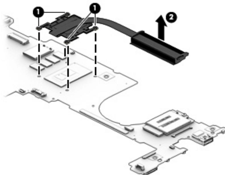
**NOTE:** The thermal material must be thoroughly cleaned from the surfaces of the heat sink and the system board each time the heat sink is removed. Thermal paste is used on the processor **(1)** and the heat sink section **(2)** that services it.
