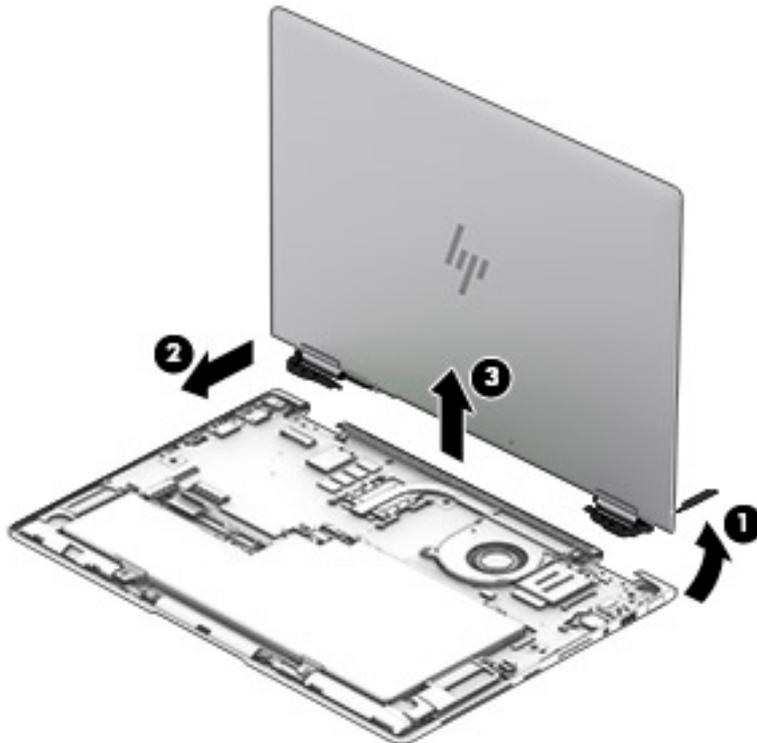
Reverse this procedure to install the display assembly.
