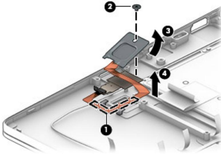
5. Remove the fingerprint reader board.
