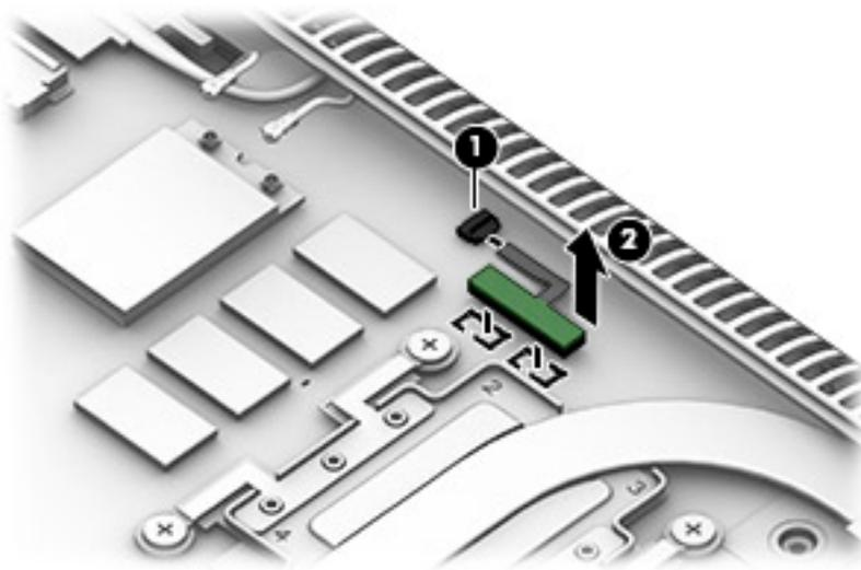
3. Remove the thermal sensor board.
